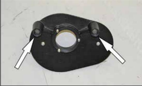
9. Install the two provided O-rings onto the filter base plate as shown.
