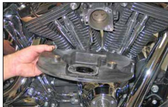
5. Remove the air filter base from the throttle body and unhook the wiring pig tail from the filter base.
