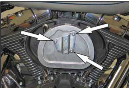
3. Remove the three bolts which secure the air filter to the filter base and then remove the air filter along with the crank case breather tubes.
