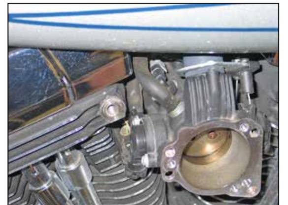
6. On Models equipped with the electrical pigtail, using the provided tie wrap, secure the wiring pig tail to the throttle body wiring harness.
