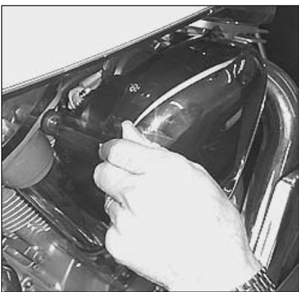
2. Remove the three air cleaner housing mounting bolts (two on top of the assembly and one on the bottom).
