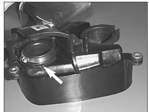
8. On 1999-2003 models install the supplied hose clamp over the air intake. Make sure the clamp is loose.
