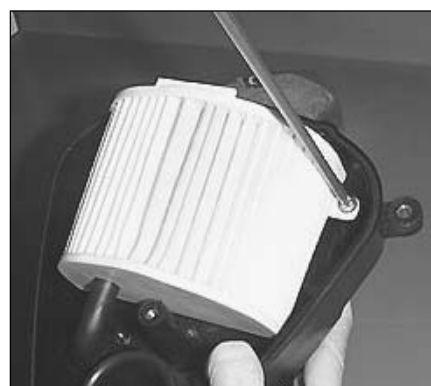
6. Remove the two screws retaining the stock air filter.
