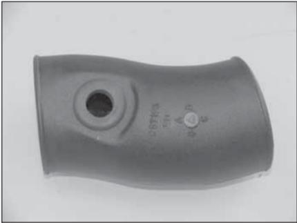
23b. On 2006 and later vehicles, install the provided grommet into the K&N® turbo inlet tube as shown.
