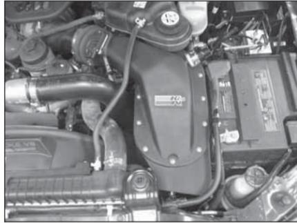
27. Install the K&N® air box lid onto the air box base making sure the silicone hose is completely installed onto the intake inlet. Install all ten air box lid mounting nuts and washers onto the lid. Once all the nuts are installed they can be tightened completely. Tighten the hose clamp, which secures the silicone hose to the throttle body.
