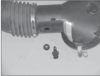
11. On vehicles equipped with an air temperature sensor, remove the air temperature sensor and grommet as shown.
