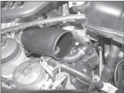
23d. On 2006 and later vehicles, install the K&N® turbo inlet tube assembly onto the turbo; rotate to align the crank case vent tube until it aligns with the vent port in the valve cover. Then snap the crank case vent tube into the valve cover and secure the tube with the provided hose clamp.
