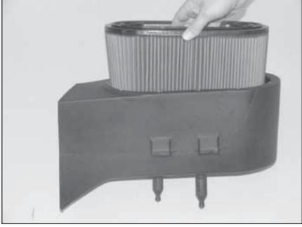
23. Install the K&N® air filter into the K&N® air box housing as shown.
