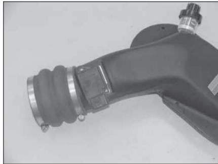
26. Install the silicone hose (08613) onto the K&N® air box lid with the provided hose clamp as shown.
