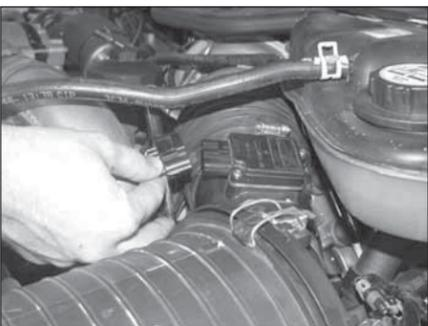
3. On vehicles equipped with a mass air sensor disconnect the mass air electrical connection as shown.
