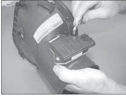
10. On vehicles equipped with a mass air sensor remove the mass air sensor from the factory air box lid with the provided torx wrench as shown.
