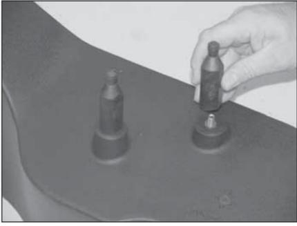
22. Install the two stand off pins onto the two studs installed in step #22.
