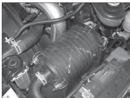
4. Release the four clamps that retains the front and back of air box.
