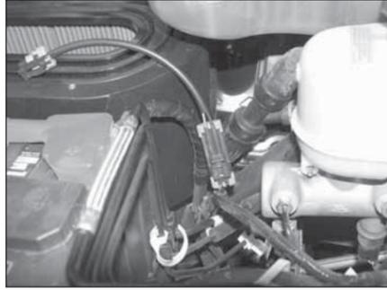
25. Install the provided wiring harness extension to the factory wiring harness filter minder connection as shown.
