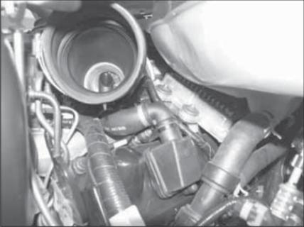
9b. On 2006 and later vehicles, using a large screwdriver, pry up on the crank case vent fitting in the valve cover to disengage it from the valve cover.
