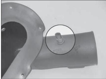
13. On vehicles equipped with the air temperature sensor, install the factory grommet and temperature sensor removed in step #11 into the K&N® intake tube at the hole drilled in step #12.
