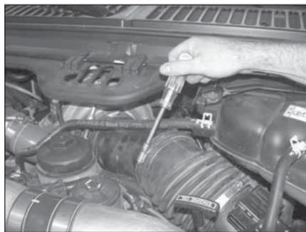
5. Loosen the hose clamp at the turbo inlet tube which secures the intake bellows as shown.
