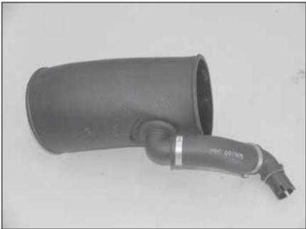
23c. On 2006 and later vehicles, install the crank case vent tube assembly removed in step #23a into the grommet on the K&N® turbo inlet tube as shown.
