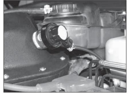
29. Connect the filter minder jumper harness into the filter minder as shown.
