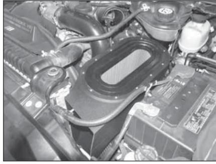
24. Install the K&N® air box base and filter into the stock location as shown.
