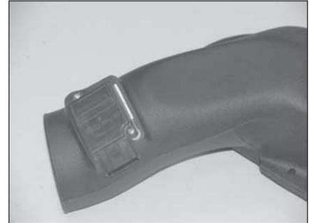
18. On vehicles equipped with the mass air sensor install the mass air sensor onto the K&N® air box lid with the provided screws and spacers as shown.
