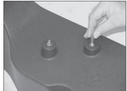
21. Install the two 8mm studs into the mounting boss on the bottom of the K&N® air box base as shown.
