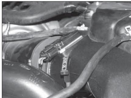
28. On vehicles equipped with a mass air sensor, connect the mass air sensor electrical connection. On vehicles equipped with an air temperature sensor, reconnect the air temperature sensor electrical connection.
