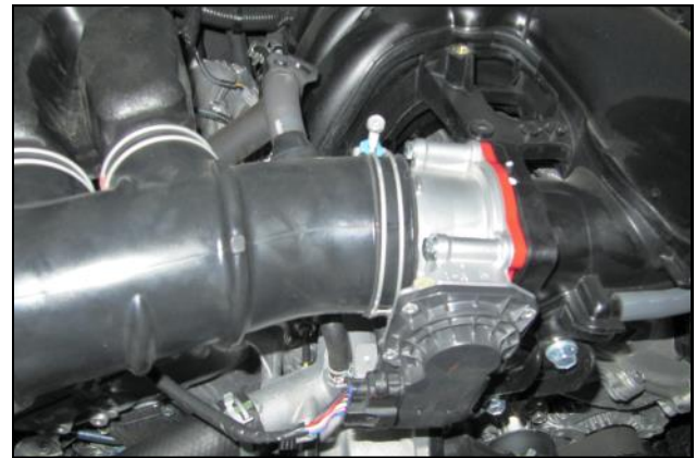
6. Reinstall the factory intake tube, tighten the two hose clamps, and reconnect the crankcase breather and Fuel pressure regulator lines. Reinstall the engine cover. Re-connect the negative battery cable!
