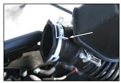
**3.** Reach down behind the engine with your pliers, and squeeze this clamp, and remove the intake tube from the throttle body.
