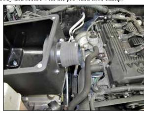
16. Install the coupler hose (084055) onto the filter adapter and secure with the provided hose clamp.
