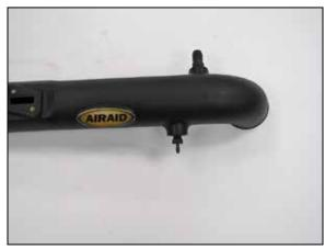
13. Install the provided vent fittings and AIRAID® decal onto the AIRAID® intake tube as shown.
