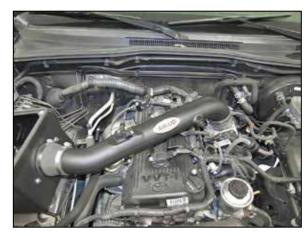
17. Install the AIRAID® intake tube into the coupler at the filter adapter and then into the coupler at the throttle body, adjust the tube for best fit and then secure with the provided hose clamps.
