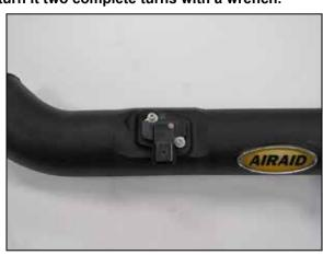
14. Remove the mass air sensor from the factory air filter housing and then install it into the AIRAID® intake tube and secure with the provided hardware.
