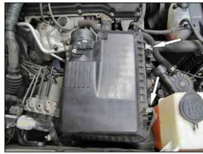
6. Release the upper air filter housing clips and remove the upper air filter housing and factory air filter.
