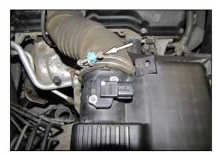
3. Loosen the hose clamp that secures the intake tube to
