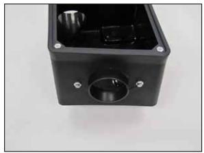
10. Install the filter adapter into the AIRAID® aid filter housing and secure with the provided hardware.
