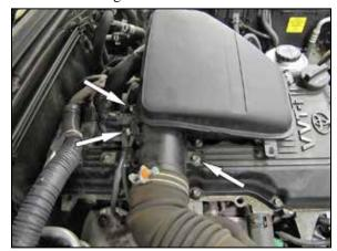
4. Remove the two bolts that secure the intake plenum to the valve cover, then remove the two bolts that secure the vacuum switching valve to the intake tube and disconnect the crank case vent hose from the valve
