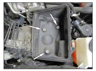
7. Remove the three bolts that secure the lower air filter housing to the inner fender.
