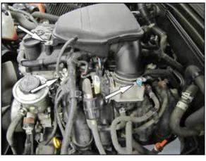
valve cover, then disconnect the vent line from the fuel pressure regulator and loosen the hose clamp securing the intake plenum to the throttle body. Remove the intake plenum from the vehicle.
