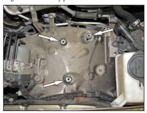
9. Install the provided rubber mounted studs into the inner fender air filter housing mounting locations.
