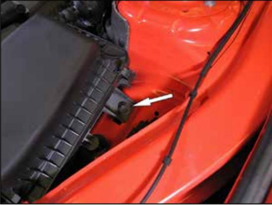
8. Remove the bolt securing the air filter assembly onto the inner fender.
