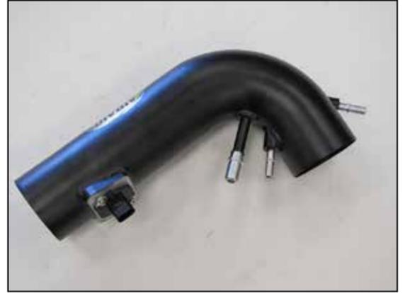
18. Remove the mass air sensor from the factory air filter housing and then install the mass air sensor into the AIRAID® intake tube and secure with the provided hardware.
