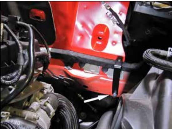
10. Install the heat shield mounting bracket (064325) onto the inner fender as shown using the provided hardware.
