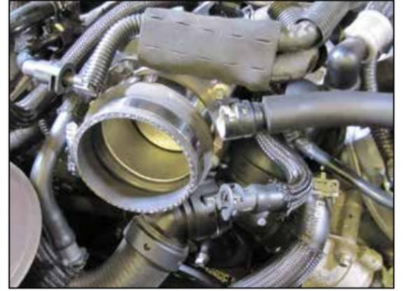
17. Install the provided hump coupler (08699) onto the throttle body and secure with the provided hose clamp.
