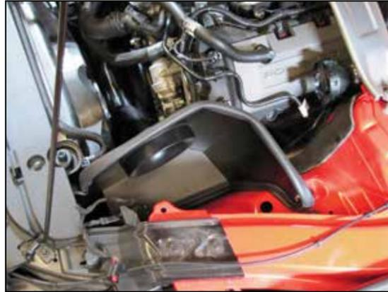
14. Set the heat shield onto the mounting bracket installed in step #10 and secure with the provided hardware.
