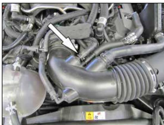
3. Depress the locking tab and then disconnect the idle bypass hose from the intake tube.
