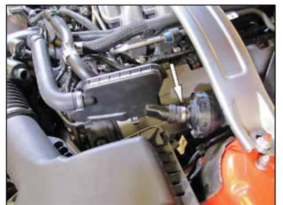
5. Cut the clamp that secures the sound tube/chamber to the sound drum and then disconnect the sound tube/chamber from the sound drum.
