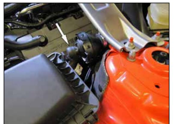
6. Install the provided cap onto the sound drum.
