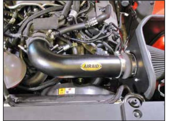
19. Install the AIRAID® intake tube into the hose at the filter adapter and then into the hose at the throttle body, adjust the tube and hoses for best fit and then secure with the provided hose clamps.
