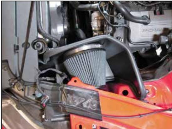
15. Install the AIRAID® air filter onto the adapter and secure with the provided hose clamp then secure the heat shield to the air filter housing mounting location using the provided hardware.
