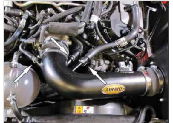
20. Connect the crank case vent, EVAP vent and idle by pass lines to the quick disconnect fittings installed into the AIRAID® intake tube.
