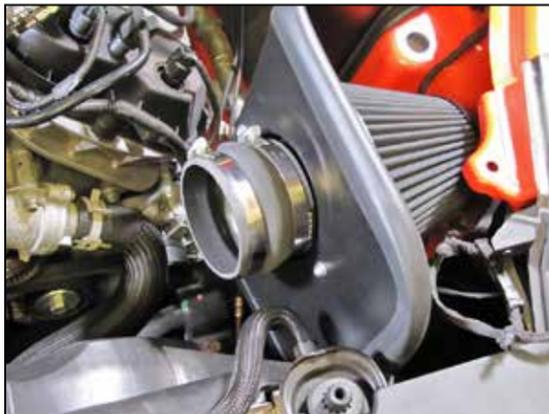
16. Install the provided hump coupler (08699) onto the filter adapter and secure with the provided hose clamp.
