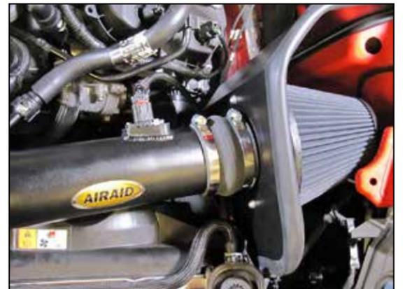
21. Connect the provided mass air sensor extension harness into the factory mass air sensor connection and then connect the other end to the mass air sensor.
