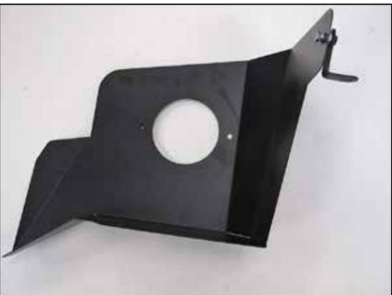
11. Install the provided heat shield mounting bracket (064326) onto the heat shield as shown using the provided hardware.
