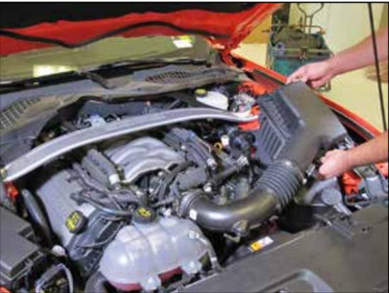
9. Loosen the hose clamp securing the intake tube to the throttle body and then remove the air filter assembly and intake tube from the engine compartment.
