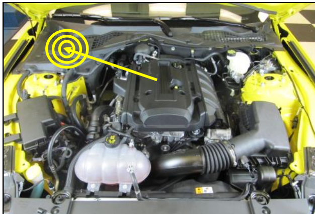
1. Remove the battery box cover in the cowl and disconnect the negative battery terminal.
