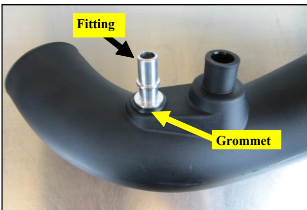
7. Insert the Grommet and Aluminum Fitting into the Airaid Intake tube as shown.
