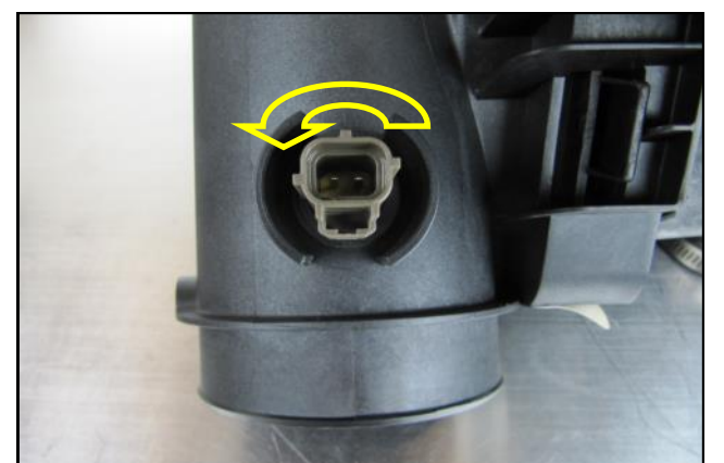
8. Tilt the air temp sensor rearward so the locking tab clears the ramp and rotate it counterclockwise 1/4 turn to release it.
