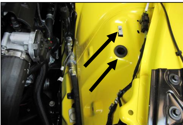
4. Be sure the speed clip and the airbox grommet remain inside the vehicle. They will be reused.
