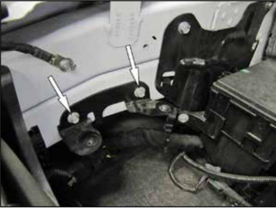
7. Remove the two bolts that secure the air filter mounting bracket to the fender and then remove the bracket from the vehicle.
