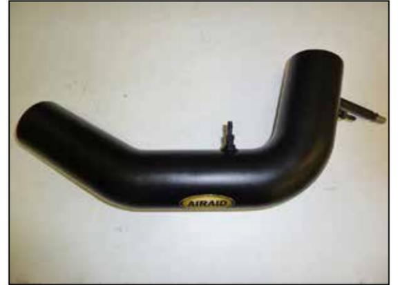
18. Install the two provided NPT vent fittings into the AIRAID intake tube as shown.
