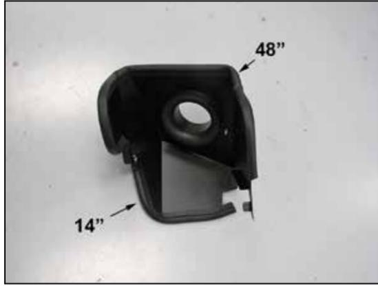
12. Install the edge trim onto the heat shield as shown.
