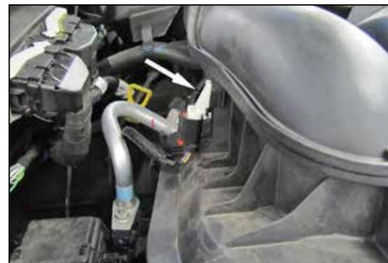
5. Unhook the wiring pigtail from the upper air filter housing.
