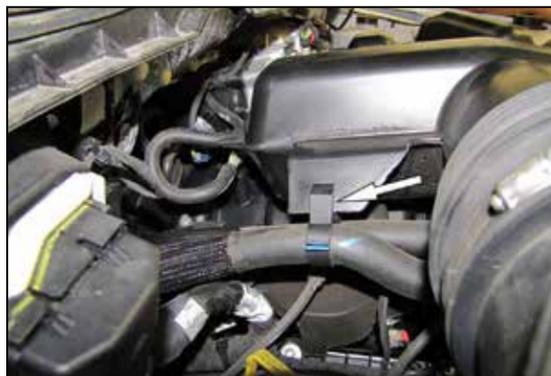
3. Disconnect the vent line from the intake plenum where shown, then unhook the heater hose clip from the intake plenum.
