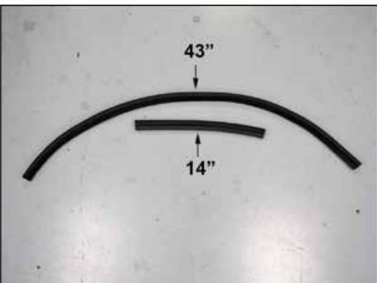
11. Cut the provided edge trim into two lengths as shown. One section should be 14" long and the other section should be 43" long.
