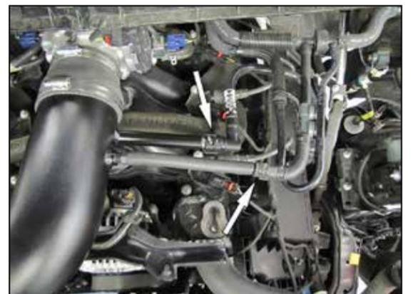
21. Install the shorter vent hose assembly onto the AIRAID intake tube and then connect the other end into the EVAP vent line.
