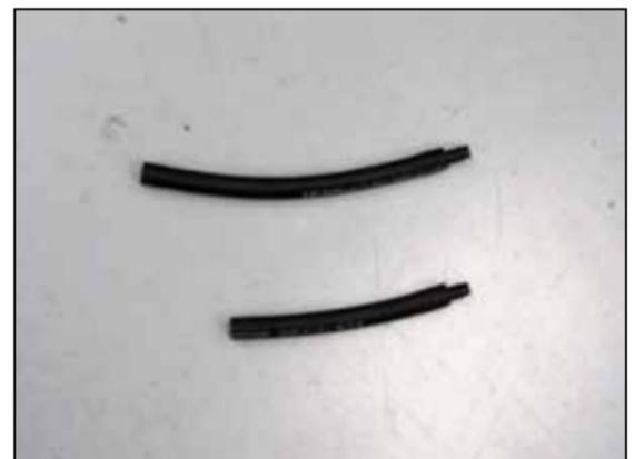
20. Install the two provided hose menders into the provided vent hoses as shown.
