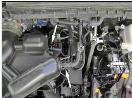
2. Release the spring clamp that secures the EVAP vent line to the intake plenum. Then release the locking tap on the Crankcase vent fitting and disconnect the crankcase vent from the intake plenum.
