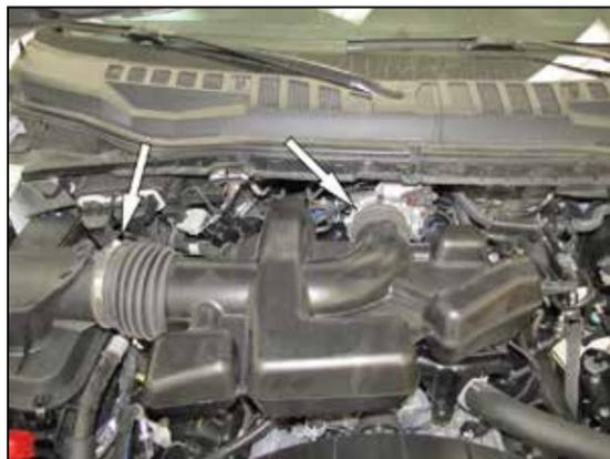
4. Loosen the hose clamps that secure the intake plenum to the air filter housing and to the throttle body, then remove the intake plenum from the vehicle.
