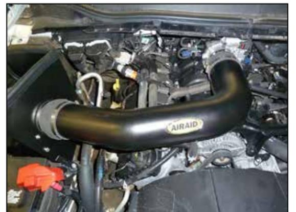
19. Install the AIRAID intake tube into the hump coupler and then into the step coupler at the throttle body, adjust the tube for best fit and then secure with the provided hose clamps.
