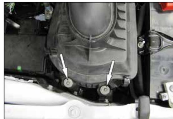
6. Remove the two bolts that secure the air filter housing to the mounting bracket and remove the air filter housing from the vehicle.
