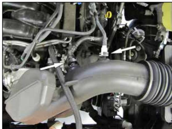
2. Disconnect the EVAP and crank case vent quick disconnect fittings.
