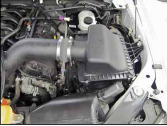
8. Install the AIRAID® intake tube into the coupler at the air filter housing and then into the coupler at the throttle body, adjust the tube for best fit and then secure with the provided hose clamps.
