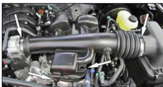
3. Unclip the harness and hose support from the intake tube. Loosen the hose clamps that secure the intake tube to the throttle body and air filter housing then remove the intake tube from the vehicle.
