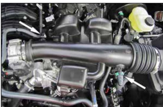
2. Release the locking tabs and then disconnect the Crank Case vent lines from the intake tube.
