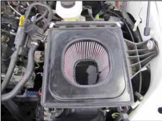
9. Install the provided AIRAID® air filter into the lower air filter housing.
