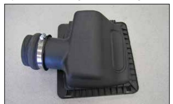
7. Install the provided hump coupler (08639) onto the air filter housing and secure with the provided hose clamp.
