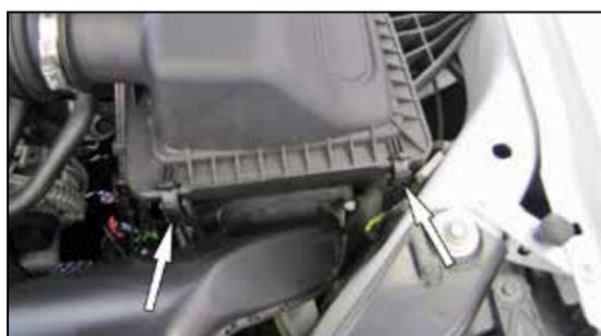
5. Release the clips that secure the upper air filter housing and then remove the upper housing and factory intake tube.
