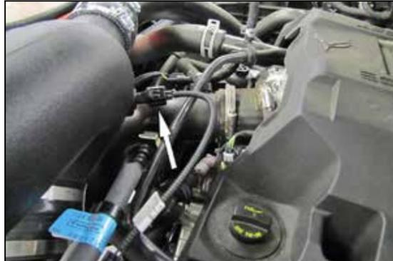
11. Reconnect the inlet air temperature sensor electrical connection.
