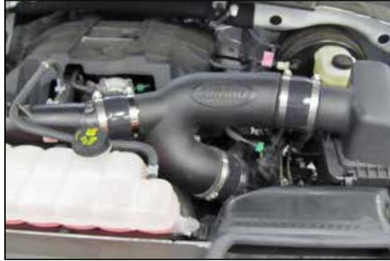
10. Install the factory upper air filter housing into the tube on the coupler and onto the lower filter housing. Secure with the factory retaining clips and hose clamp provided.
