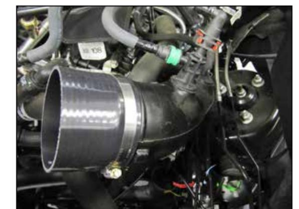
6. Install the provided coupler hose onto the turbo inlet tubes and secure with the provided hose clamps.
