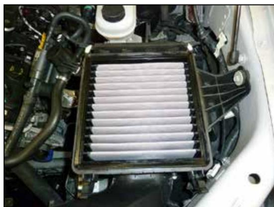
5. Install the provided AIRAID® air filter into the lower air filter housing.
