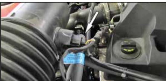
2. Disconnect the inlet air temperature sensor.
