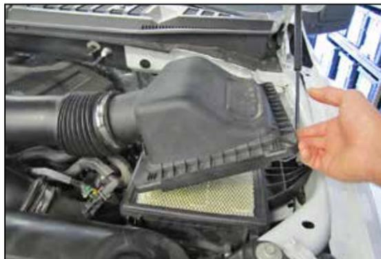
4. Release the locking clamps, lift up the upper air filter housing and then remove it from the vehicle, then remove the factory air filter.
