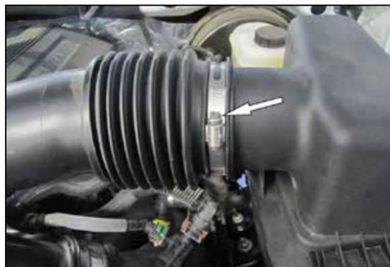
3. Loosen the hose clamp that secures the factory intake tube to the upper air filter housing.
