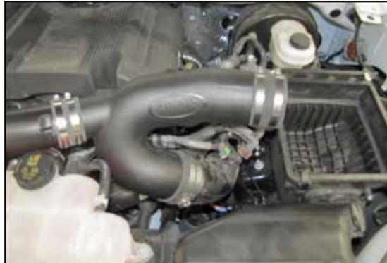
12. Install the AIRAID intake tube onto the turbo inlet tubes and secure with the provided hose clamps.
