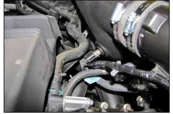
15. Reconnect the inlet air temperature sensor electrical connection.
