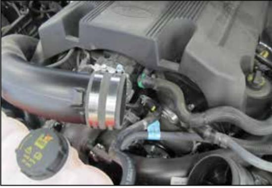
8. Install the provided coupler hose (08711) onto the passenger side turbo inlet tube and secure with the provided hose clamp.
