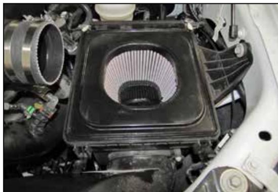
13. Install the AIRAID air filter into the lower air filter housing.
