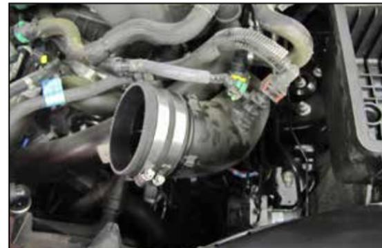
7. Install the provided coupler hose (08761) onto the driver's side turbo inlet tube and secure with the provided hose clamp.
