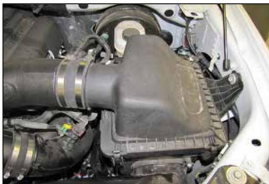
14. Reinstall the upper air filter housing onto the lower housing and into the coupler on the intake tube. Secure the housing to the lower housing with the factory clips and to the intake tube with the provided hose clamp.
