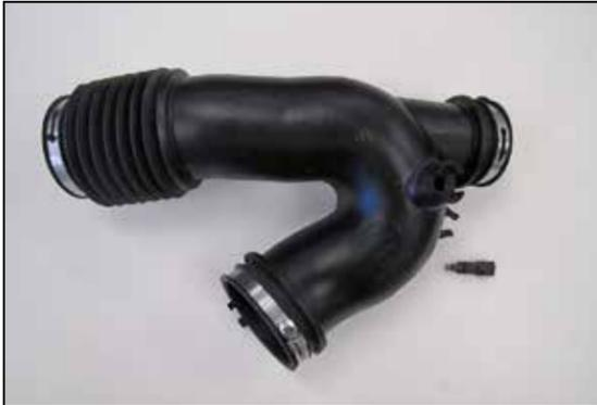
9. Remove the inlet air temperature sensor from the factory intake tube and remove the O-Ring from the sensor.
