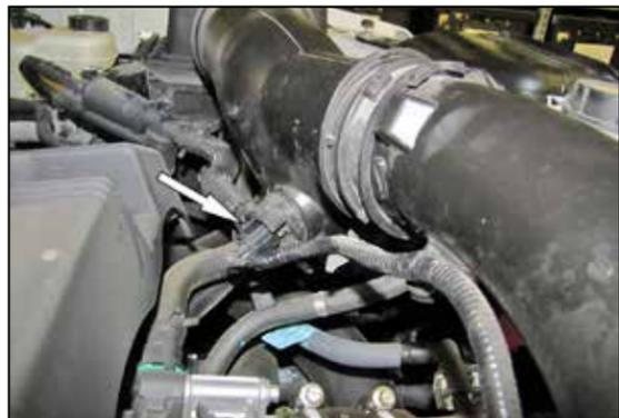
2. Disconnect the inlet air temperature sensor electrical connection.
