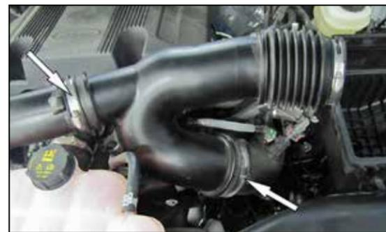
5. Loosen the two remaining hose clamps that secure the factory intake tube to the turbo inlet tubes and then remove the intake tube from the vehicle.
