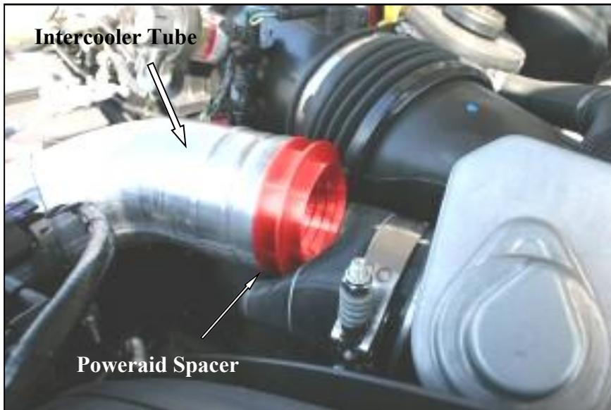
2. Install the larger diameter end of the Poweraid Spacer into the aluminum intercooler tube as shown. Next reinstall the coupler over the spacer, and onto the intercooler tube in the factory position. Slide the hose clamp back up the tube and reposition it in the original position over the coupler and tighten to the manufacturer's specifications.
