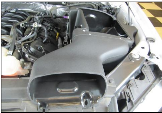
10. Place the Airaid air Box/Inlet assembly into the inner fender area of the vehicle as shown.
