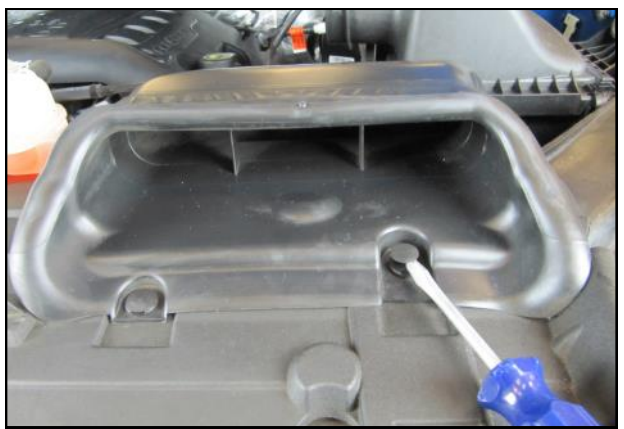
4. Using a standard blade screwdriver, gently pry up the center posts of the plastic rivets in the air inlet and remove them.
