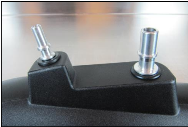
14. Gently insert the Aluminum Breather Fittings into the Grommets. Hint: Soapy water makes for a good Grommet lube .
