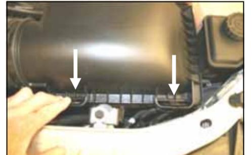
**3. Pull both lockdown tabs towards you on the factory airbox lid to remove the lid from the base.**
