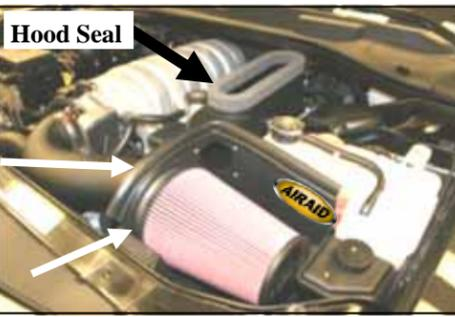
**17.** Install the Airaid Premium Filter (#1), onto the filter adapter inside of the CAD, and tighten the hose clamp. Next install the weather strip (#9) onto the top of the CAD. Apply the hood seal onto the top side of the Hood Scoop (recommended to prep surface with alcohol for permanent bond).
