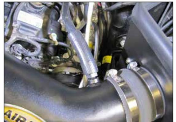
21. Install the provided crank case vent hose onto the fitting installed into the AIRAID® intake tube and then connect the other end to the factory crank case vent tube.
