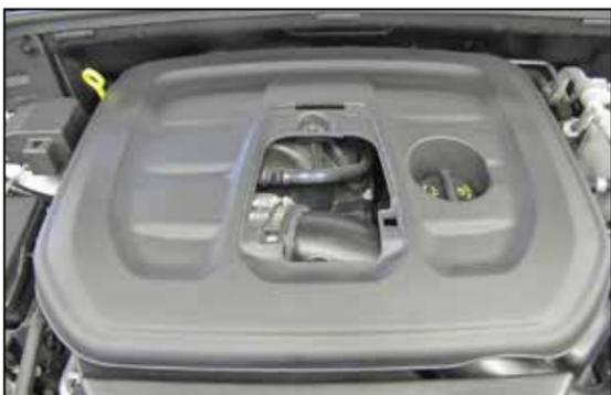
2. Lift up the inspection cover and remove the bolt that secures the decorative engine cover. Then remove the decorative engine cover from the vehicle.
