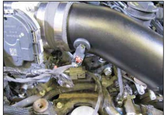
20. Reconnect the inlet air temperature sensor electrical connection.
