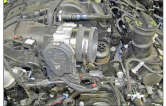
18. Install the provided step coupler onto the throttle body and secure with the provided hose clamp.
