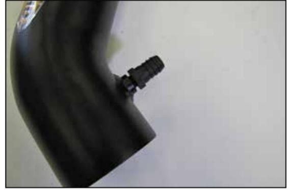
17. Install the provided vent fitting into the AIRAID® intake tube as shown.
