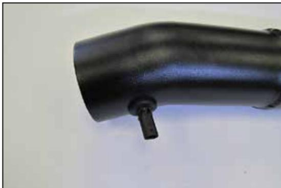
16. Install the provided grommet into the AIRAID® intake tube, then remove the O-Ring from the inlet air temperature sensor and then install the sensor into the grommet installed into the AIRAID® intake tube.
