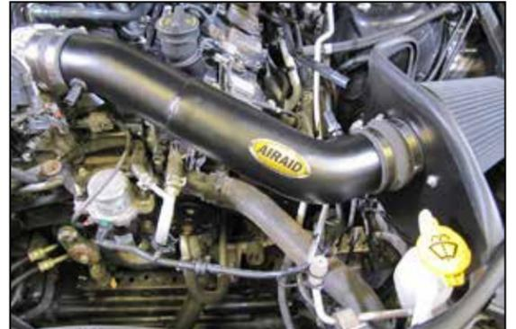
19. Install the AIRAID® intake tube into the coupler at the throttle body and then into the hump coupler, adjust the tube for best fit and then secure with the provided hose clamps.
