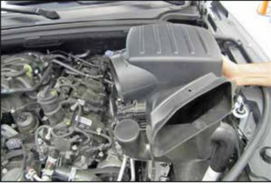
7. Lift up the air filter housing to dislodge it from the mounting grommets and then remove it from the vehicle.
