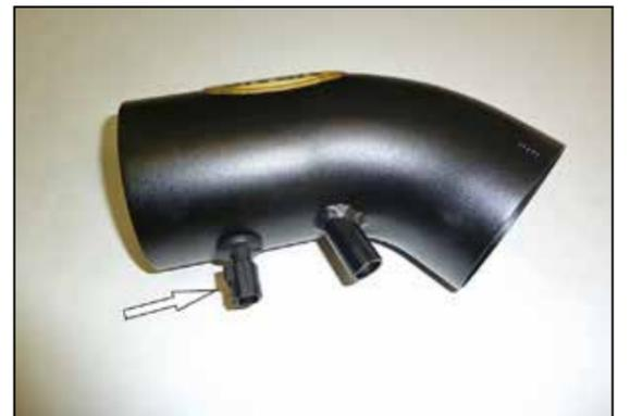
20. Install the provided grommet into the AIRAID® intake tube. Remove the O-ring from the inlet air temperature sensor and then install the sensor into the grommet as shown.
