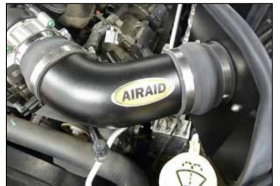
21. Install the AIRAID® intake tube into the hump coupler and then into the straight coupler, adjust the intake tube for best fit and then secure with the provided hose clamps.
