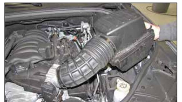
6. Lift up the air filter assembly to dislodge it from the mounting grommets and the remove the complete assembly from the vehicle.
