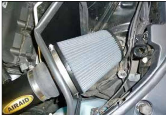
25. Install the AIRAID® air filter and secure with the provided hose clamp.
