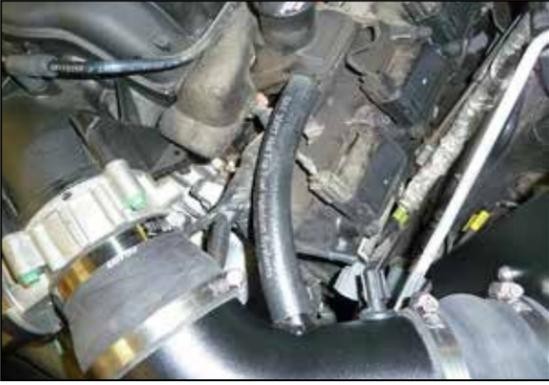
22. Install the provided crank case vent hose onto the valve cover port and then to the port on the AIRAID® intake tube.
