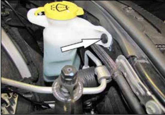
8. Remove the retaining clip that secures the windshield washer bottle to the core support.
