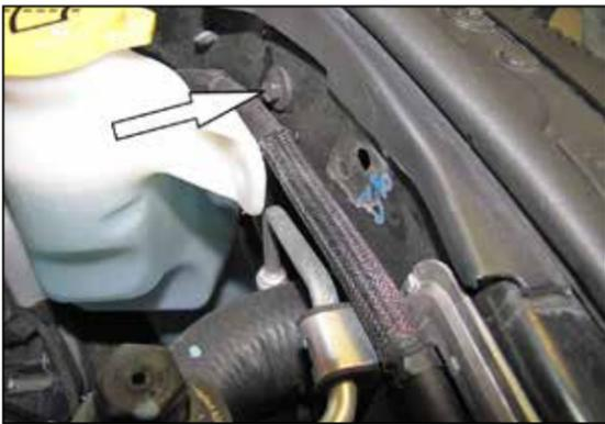
9. Remove the core support bolt shown.
