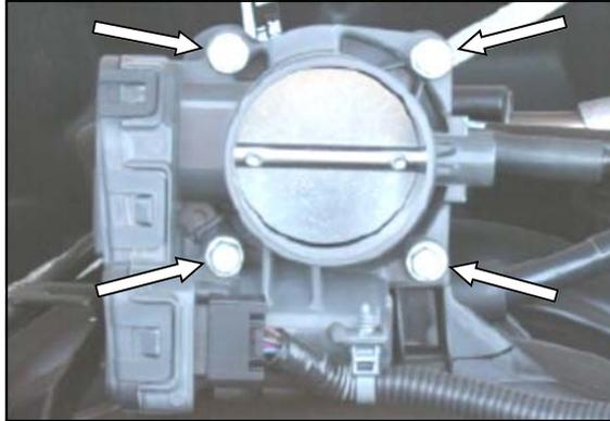
3. Using a 10mm socket, remove the four bolts that secure the throttle body to the intake manifold. Next, rotate the factory throttle body out of the way to allow access to the intake manifold. Make sure the factory blue gasket is seated in the groove on the intake manifold.
