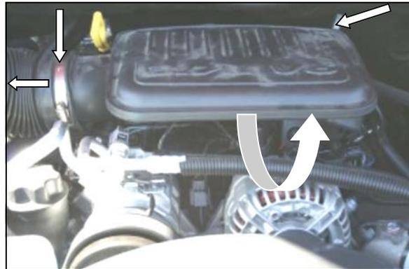
**2. All other listed vehicles:** Using a 5/16" socket, or flat blade screwdriver, loosen the hose clamp which secures the factory intake tube to the resonator box. Disconnect the factory temperature sensor wiring harness from the sensor in the resonator box. Slide the factory intake tube off of the resonator box. Remove the resonator box by pulling straight forward to release it from the throttle body and the grommet mounts. Save the resonator box for reuse.
