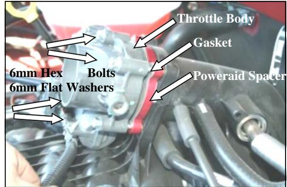
4. Install the Poweraid Spacer (#1) with the bore extending into the intake manifold. Install the Gasket (#2) between the Poweraid Spacer and the throttle body. Install four 6mm x 50mm hex bolts (#3) and 6mm flat washers (#4) through the throttle body, Poweraid Spacer, Gasket, and into the intake manifold. Using a 10mm socket, tighten all four throttle body bolts evenly, to the manufacturer's specifications. **Do Not Over Tighten The Bolts!** Reference picture below for spacer orientation.
