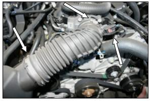
1. Disconnect the negative battery cable! Loosen 2 hose clamps on each end of the factory intake tube. Slide the red locking tab, and then squeeze the black tab, and disconnect the intake tube temperature sensor wiring harness. Remove the tube from the vehicle.
