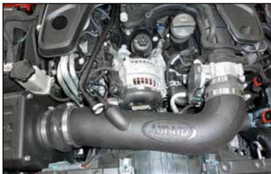
14. Install the intake tube into the hump coupler and then into the coupler at the throttle body, adjust the tube for best fit and secure with the provided hose clamps.
