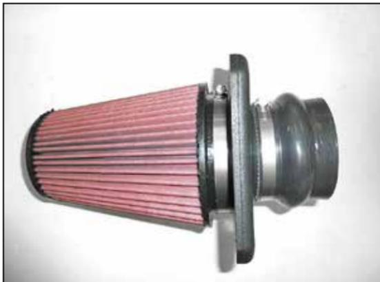
10. Install the air filter and hump coupler onto the filter housing side panel as shown and secure with the provided hose clamps.
