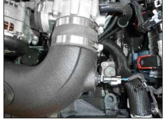
15. Reconnect the inlet air temperature sensor electrical connection.
