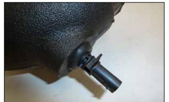
6. Install the provided grommet into the AIRAID® intake tube. Remove the inlet air temperature sensor from the factory intake tube, Remove the O-ring from the sensor and then install the sensor into the grommet installed into the AIRAID® intake tube.
