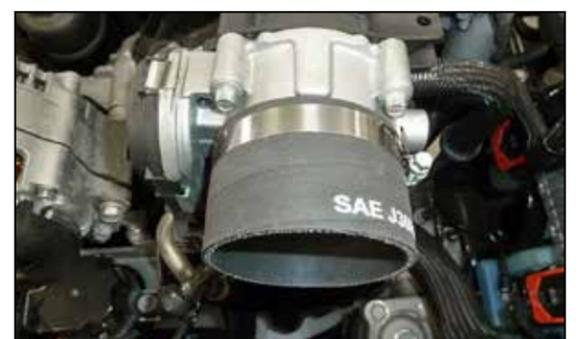
5. Install the provided coupler hose onto the Throttle body and secure with the provided hose clamp.
