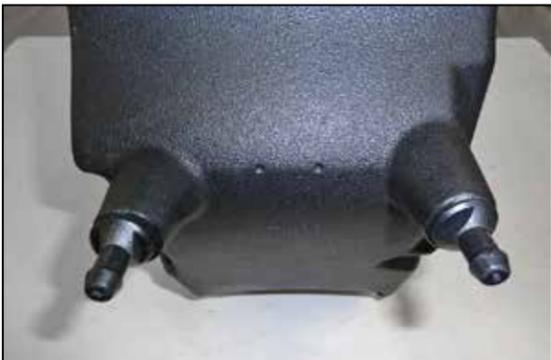
9. Install the two provided mounts onto the bottom of the air filter housing using the provided hardware.
