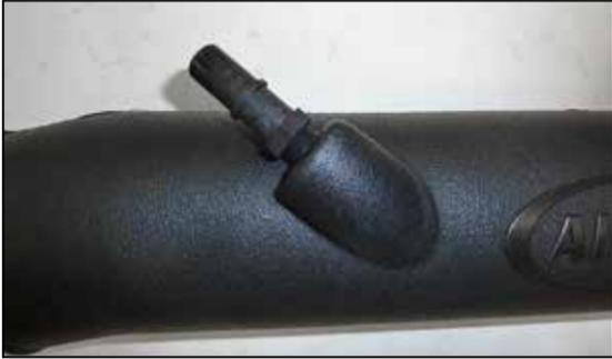
7. Install the provided quick disconnect vent into the AIRAID® intake tube as shown.
