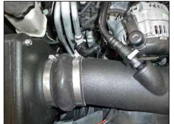
16. Connect the factory crank case vent hose to the quick disconnect fitting installed into the AIRAID® intake tube.
