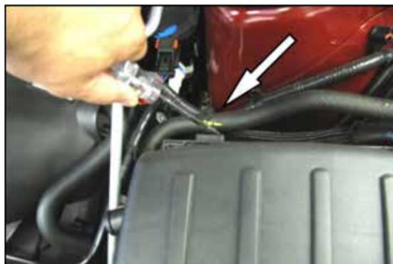
3. Using a standard head screwdriver, carefully pry and separate the hose anchor from the airbox lid. This anchor will be reused on the Airaid Intake System.
