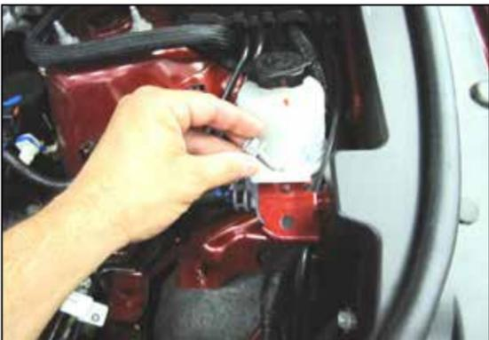
12a. On vehicles equipped with a power steering reservoir on the inner fender, remove the bolt securing the reservoir and set aside. This bolt will be reused in a later step to hold the Mounting bracket.
