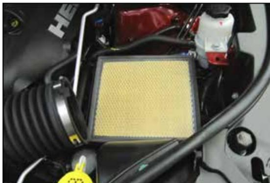
4. Remove the upper half of the airbox and the factory air filter.
