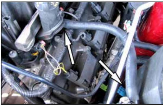
14. On V8 motors, replace the factory crankcase breather line with the 13" Breather Hose (#5) and connect it to the Airaid Intake Tube. Disregard the 90 deg. Elbow (#7) it will not be used.
