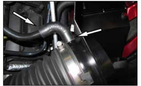
15. On V6 motors, connect the factory crankcase breather hard line to the Airaid Intake Tube using the 90 deg. Breather Elbow (#7). Disregard the 13" Breather Hose (#6) it will not be used.
