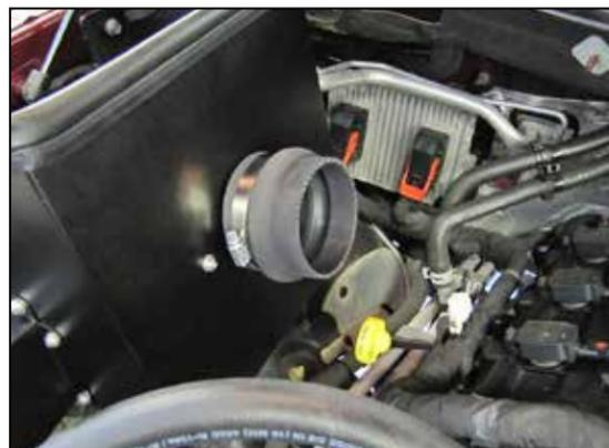
16. Install the provided coupling hose (08699) onto the filter adapter and secure with the provided hose clamp.
