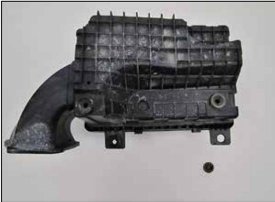
10. Remove one of the rubber mounting grommets from the factory air box.
