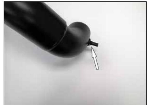
20. Install the inlet air temperature sensor into the grommet installed into the intake tube.
