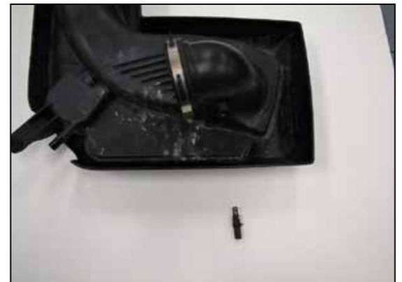
19. Remove the inlet air temperature sensor from the factory intake plenum.
