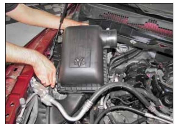
6. Lift the air box assembly off of the mounting studs and then remove the air box from the vehicle.
