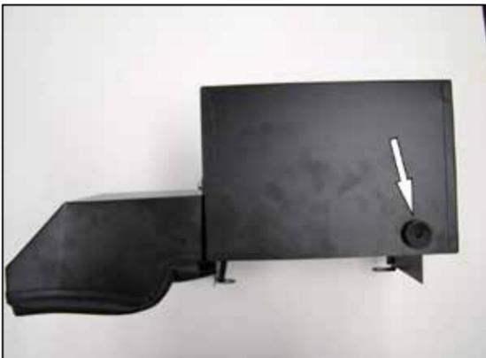
11. Install the factory rubber mounting grommet into the AIRAID heat shield as shown.
