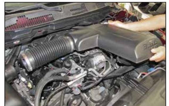
5. Lift up the intake plenum to dislodge it from the mounting grommets and then remove the plenum from the vehicle.
