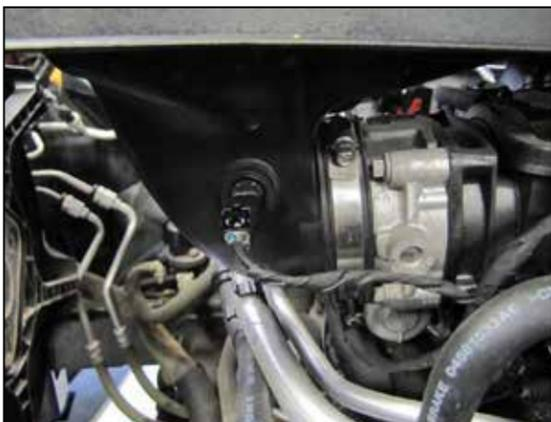
2. Disconnect the Inlet air temperature sensor electrical connection and loosen the hose clamp securing the intake plenum to the throttle body.
