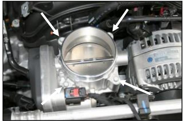
2. Remove the four bolts that secure the throttlebody to the intake manifold. Without disconnecting the wiring harness, remove the throttlebody from the intake manifold and set it aside.
