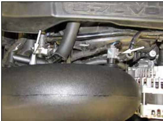
14. Connect the factory crank case vent hose to the quick disconnect fitting installed into the AIRAID® intake tube. Reconnect the inlet air temperature sensor electrical connection.
