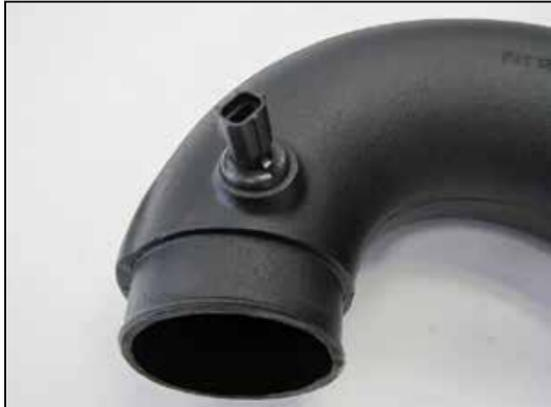
12. Install the inlet air temperature sensor into the AIRAID® intake tube using the provided grommet.
