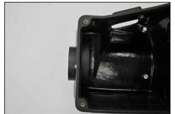
5. Install the filter adapter into the AIRAID® air filter housing and secure with the hardware provided.
