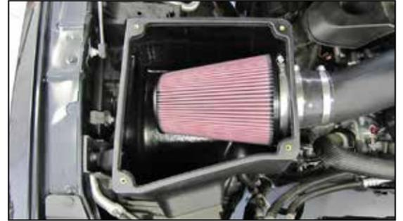
15. Install the AIRAID® air filter onto the filter adapter and secure with the provided hose clamp.
