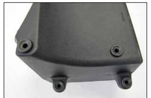
6. Remove the mounting grommets from the factory air filter housing and install them into the AIRAID® filter housing as shown.
