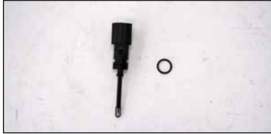
11. Remove the inlet temperature sensor from the factory intake tube and then remove the O-ring from the sensor.
