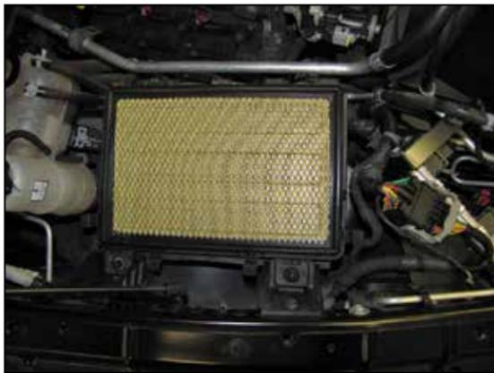
5. Lift the lower air filter housing up and then remove the housing from the vehicle.
