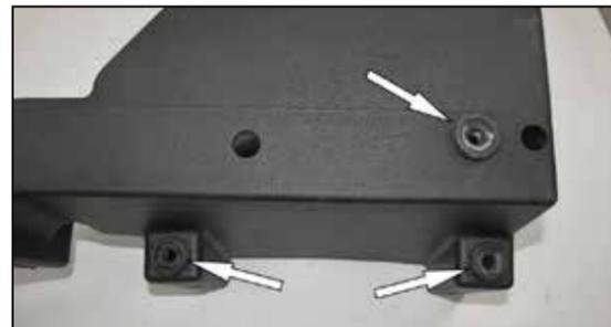
8. Remove three of the factory mounting grommets from the factory air filter housing and install them as shown into the AIRAID air filter housing.
