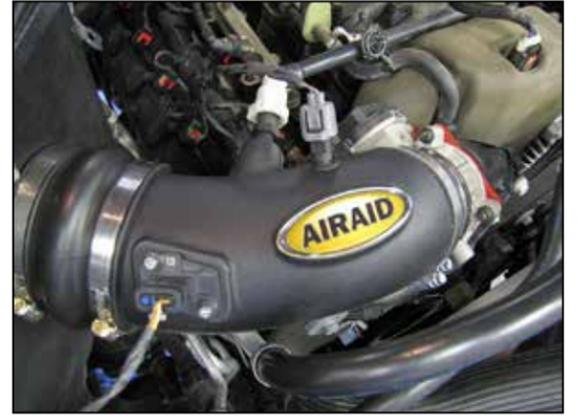
16. Connect the crank case vent to the fitting installed into the AIRAID intake tube. Reconnect the mass air sensor and inlet air temperature sensor electrical connections.
