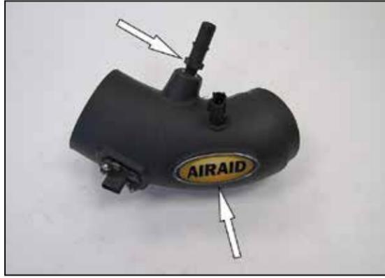
12. Install the provided quick connect vent fitting and AIRAID decal onto the AIRAID intake tube as shown.
