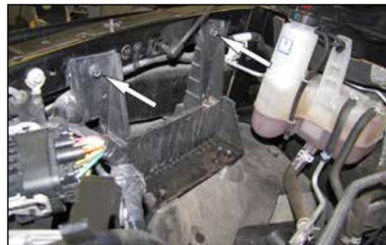
6. Remove the two upper filter housing bracket mounting bolts.
