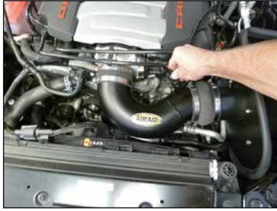
25. Connect the crank case vent hose to the quick disconnect fitting installed into the AIRAID® intake tube.
