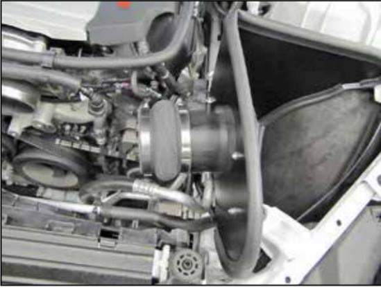
22. Install the provided step hump coupler (08633) onto the filter adapter and secure with the provided hose clamp.
