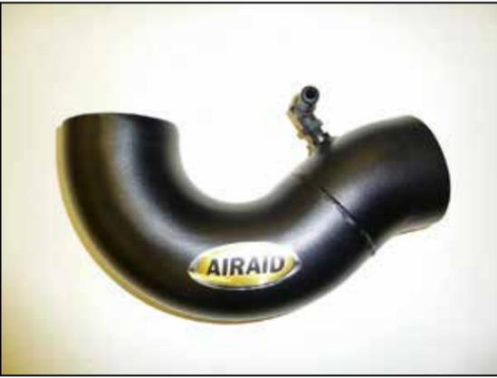
23. Install the provided 90° fitting into the AIRAID® intake tube as shown.
