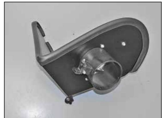
19. Install the mass air sensor into the AIRAID® mass air adapter and secure with the provided hardware.
