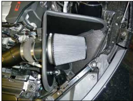
27. Install the AIRAID® air filter and secure with the provided hose clamp.
