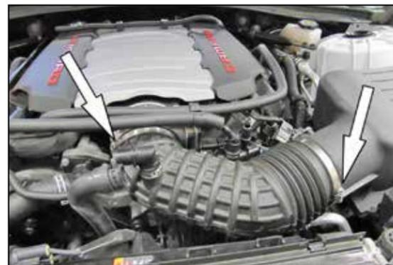
5. Loosen the hose clamps securing the intake tube to the throttle body and air filter housing and then remove the intake tube.
