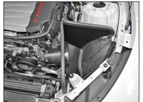
20. Install the AIRAID® heat shield assembly onto the air filter housing mounting grommets.
