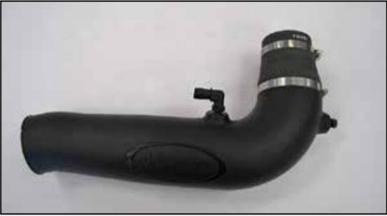
8. Install the provided step coupler (084104) onto the AIRAID® intake tube as shown.
