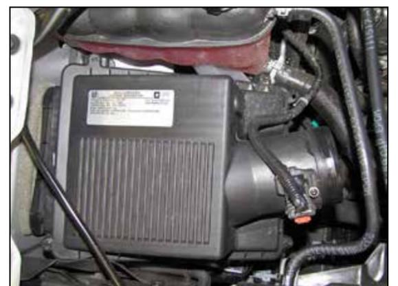
5. Loosen the four screws that secure the upper air filter housing and then remove the upper housing and set to the side.
