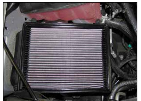
6. Replace the factory air filter with the provided AIRAID® air filter and reinstall and secure the upper air filter housing.
