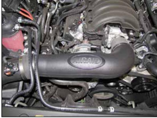
10. Install the AIRAID® intake tube into the coupler on the air filter housing and then onto the throttle body, adjust the tube for best fit and then secure with the provided hose clamps.
