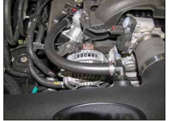
12. Connect the Crank case vent hose quick connect fitting onto the valve cover port and then connect the open end to the fitting installed into the intake tube and secure the hose clamps.
