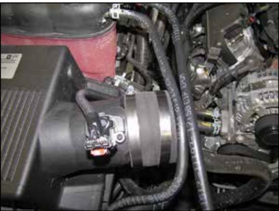
9. Install the provided coupler (08760) onto the factory air filter housing as shown.
