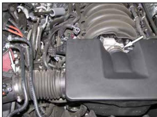
4. Loosen the hose clamps securing the intake plenum to the throttle body and air filter housing then remove the intake plenum from the vehicle.
