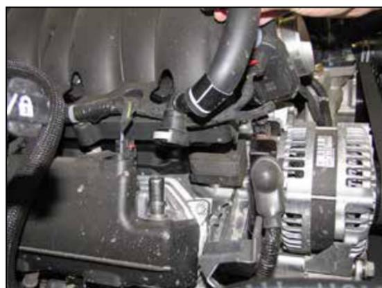
3. Rotate the crank case vent hose to access the quick connect release tap and then disconnect the crank case vent hose from the valve cover port.
