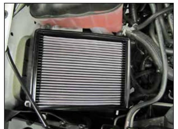
5. Install the AIRAID® air filter into the lower filter housing and then reinstall the upper housing and secure with the factory hardware.
