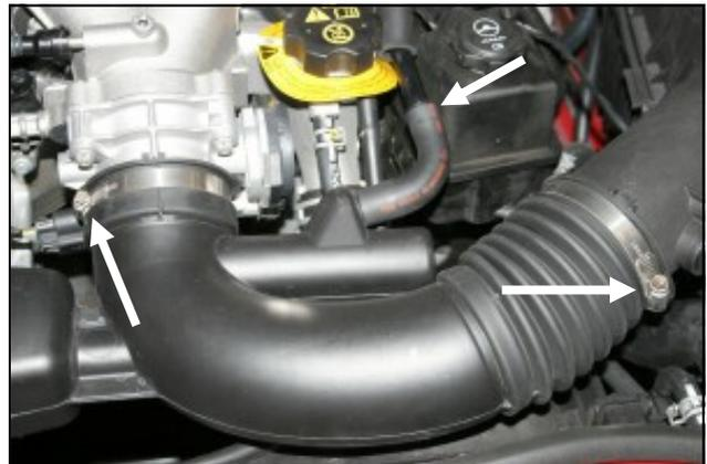
**2.** Disconnect the breather hose elbow at the hard plastic breather tube. Loosen the two hose clamps that secure the intake tube to the throttlebody, and the air cleaner lid.
