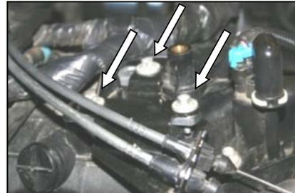
8. **If you have an electronic throttlebody, (no cables) skip to step #10.** Re-install the throttle cable bracket and the 3 factory bolts removed in step 4. Some minor adjustments to the extension plates may be necessary to get all three bolts to be aligned in position.
