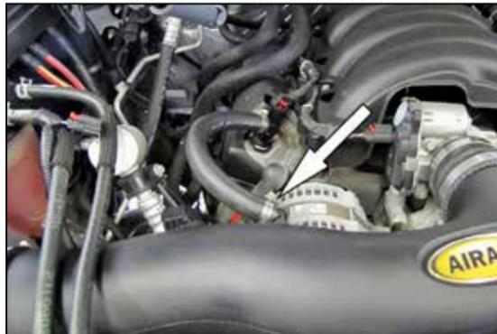
11. Install the provided PCV hose onto the fitting on the valve cover and in the intake tube with the provided hose clamps. Secure the PCV hose with the hose clamps.
