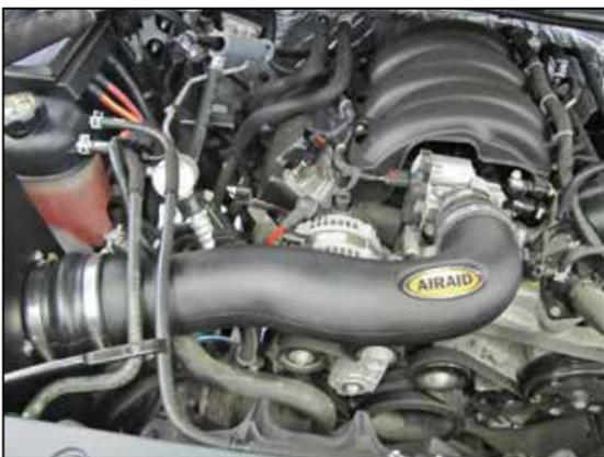
9. Install the AIRAID® intake tube into the hump coupler and then into the step coupler, adjust the tube and couplers for best fit and then secure all the hose clamps.
