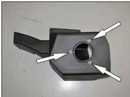
4. Install the filter adapter into the AIRAID® air box and secure with the provided hardware.
