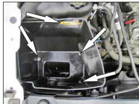
5. Install the AIRAID® air box into the vehicle and secure with three of the OEM bolts from step #3. Apply one of the provided AIRAID® decals to the air box as shown.
