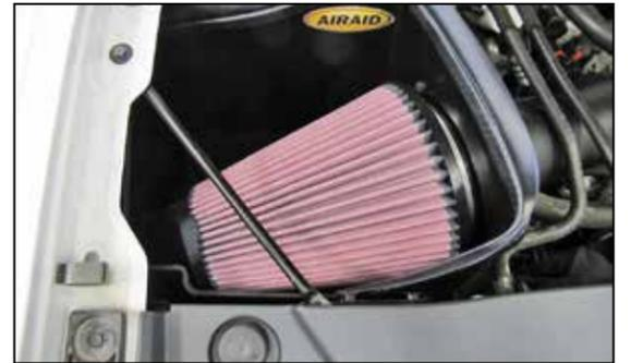
15. Rotate the fender brace back into position and reinstall the factory bolt and tighten the core support bolt.
