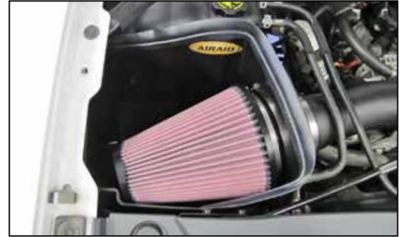
14. Install the weather strip onto the top edge of the AIRAID® air box with the contour rolling away from the filter as shown.
