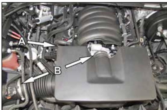
1. **Disconnect the negative battery cable!** A. Depress the grey locking tab in the PCV breather connector quick disconnect fitting on the valve cover and disconnect the PVC from the valve cover. B. Loosen the hose clamps that secure the intake plenum assembly to the throttle body and air filter housing and then remove the complete assembly from the vehicle.
