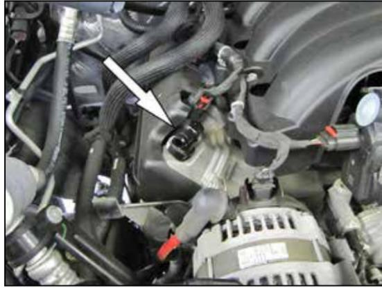
10. Install the provided 90° quick disconnect fitting onto the valve cover PCV port.
