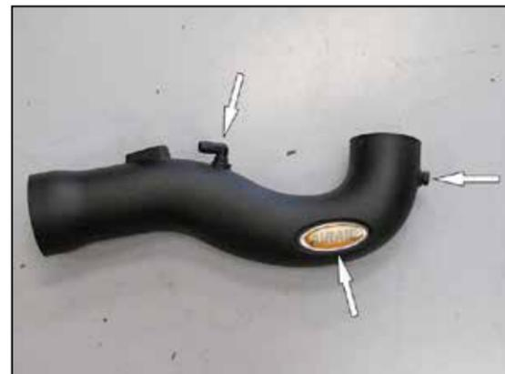
6. Install the 3/8" NPT elbow fitting and 3/8" NPT plug into the AIRAID® intake tube where shown. Apply the provided AIRAID® decal onto the intake tube where shown. **NOTE: Plastic NPT fittings are easy to cross thread. Install the vent fitting "hand" tight, then turn it two complete turns with a wrench.**
