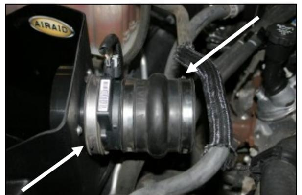
**9. Reinstall the MAF sensor and coupler onto the filter adapter and tighten the clamp. Next install the hump hose (#5) onto the MAF using two #60 hose clamps (#13). Leave these two clamps loose for now.**
