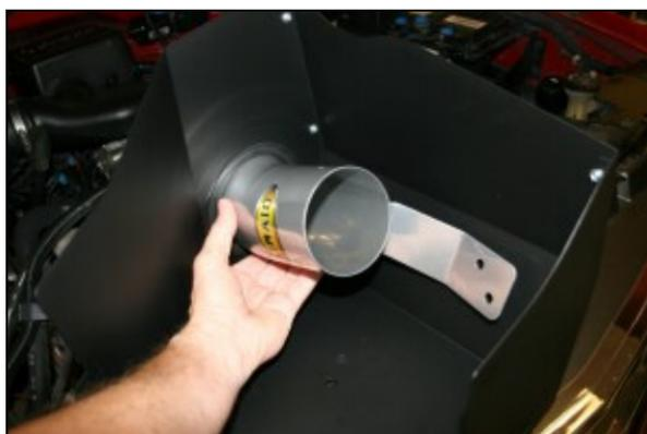
5. Insert the air intake tube that was removed in step #1 thru the hole in the MAF panel and then rotate it clockwise so that the holes in the bracket on the tube line up with the two holes in the bottom panel.
