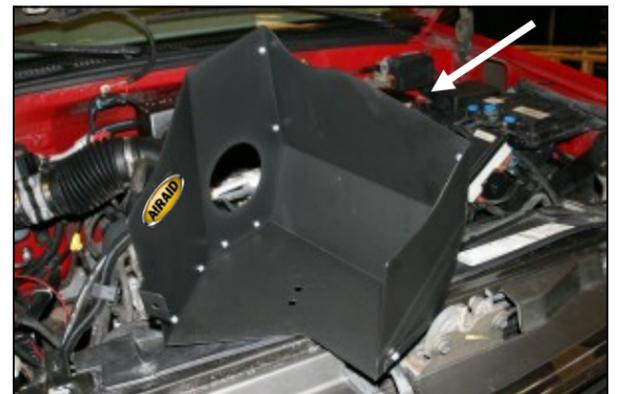
3. Assemble the three Cold Air Dam (CAD) panels (#s 2, 3, &4) as shown using nine 6-32 screws (#8), nine #6 washers (#7), and nine nuts (#9). Apply the Airaid Foil Decal onto the Panel as shown.
