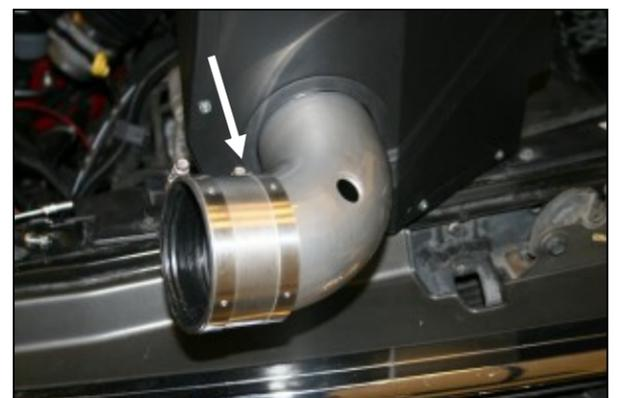
6. Install the stainless steel coupler removed in step #1 onto the air intake tube and tighten *only* the hose clamp on the tube.
