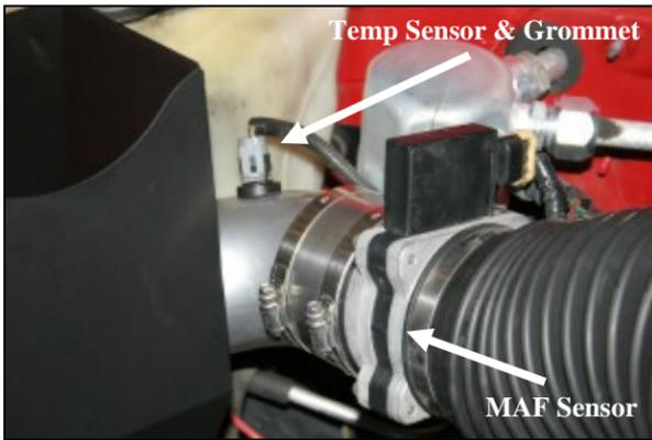
8. Connect the MAF sensor to the stainless steel coupler and tighten the hose clamp. Install the factory grommet removed in step #1, into the hole in the Airaid intake tube. **VERY CAREFULLY** install the factory temperature sensor into the grommet.
