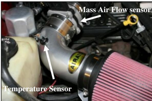
1. **Disconnect the negative battery cable. VERY CAREFULLY!** Remove the air intake temperature sensor first, and then the grommet from the air intake tube and set them aside. . Loosen the two hose clamps on the stainless steel coupler that connects the air intake tube to the Mass Air Flow (MAF) sensor. Loosen the hose clamp on the air filter and remove it from the vehicle.
