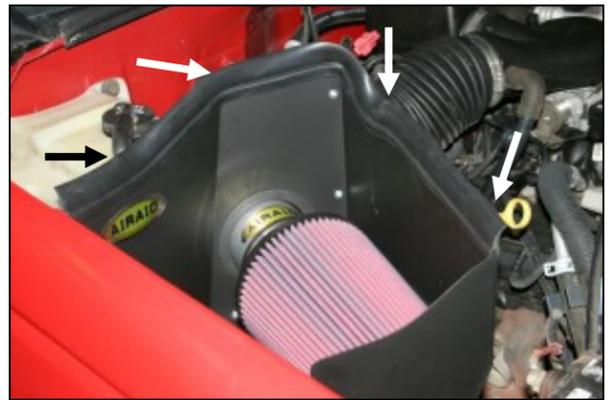
9. Install the Airaid Premium Filter (#1) onto the Airaid intake tube as shown, and then tighten the hose clamp. Next, install the weather strip on top of the CAD, starting at the right fender working your way towards the front of the vehicle.
