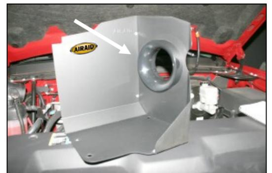
**9.** Assemble the Cool Air Dam panels (CAD) (#2 & #3) using five 6-32 x 5/16" screws (#10), #6 flat washers (#11), and 6-32 keps nuts (#12). Next install the air filter adapter (#5) into the panels as shown using three 1/4 - 20 x 1/2" button head bolts (#13), and 1/4" flat washers (#14). Apply the Airaid Decal as shown.
