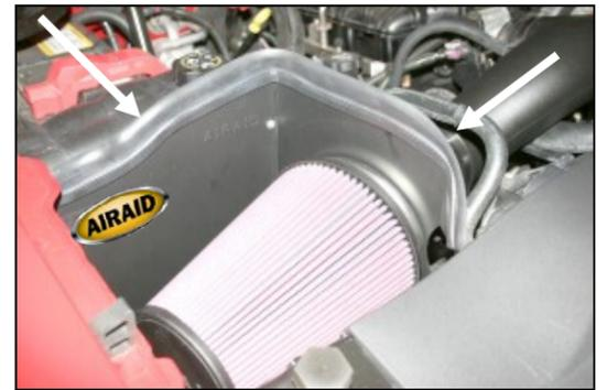
**15.** Install the Airaid Premium Filter (#1) onto the air filter adapter, and tighten the hose clamp. Next install the provided weather strip (#9) onto the top of the CAD. *For ease of install, start at the inner fender, and work your way towards the radiator.* Reinstall the beauty cover.
