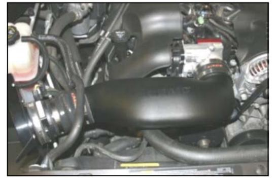
**12.** Install the Modular Intake Tube into the hump hose first, and then into the throttle body. Adjust for fit, and tighten all four hose clamps. Re-insert the plastic piece from step #3 into the hole on the bottom of the MIT.
