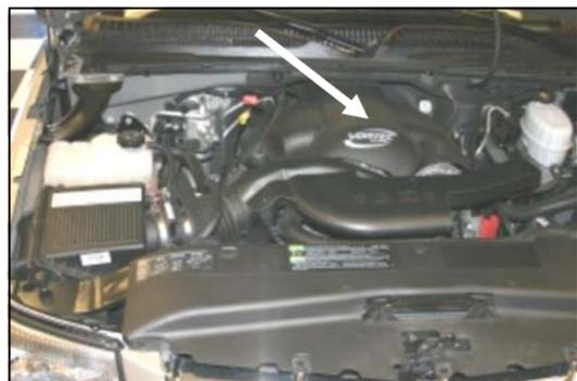
1. **Disconnect negative battery cable.** With a 5/16" socket, remove one bolt from the top of the beauty cover. Set the bolt and the cover aside for re-installation later.
