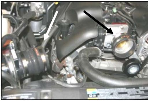
**11.** Install the urethane hump hose (#6) on the Mass Air Flow sensor with two #60 hose clamps (#15). Next install the coupler (#7) on the throttle body with two #64 hose clamps (#16).
