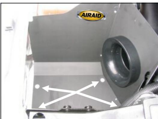
**7.** Install the Airaid Cool Air Dam assembly in the engine compartment using four M6-1x25 hex bolts (#14) and 1/4" flat washers (#13). Apply the Airaid Foil Decal onto the Panel as shown.
