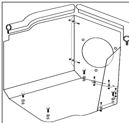
**5.** Assemble the Airaid Cool Air Dam panels (#2, #3) using five 6-32 x 5/16" screws (#9), #6 flat washers (#10) and 6/32 keps nuts (#11).
