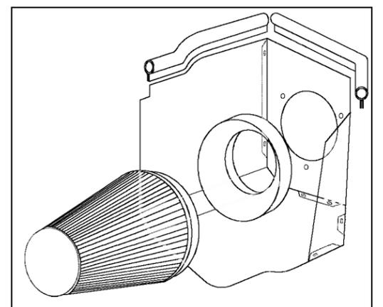
**6.** Using three 1/4-20 x 1/2" button head bolts (#12) and 1/4" flat washers (#13), install the filter adapter (#4) onto the Airaid Cool Air Dam.
