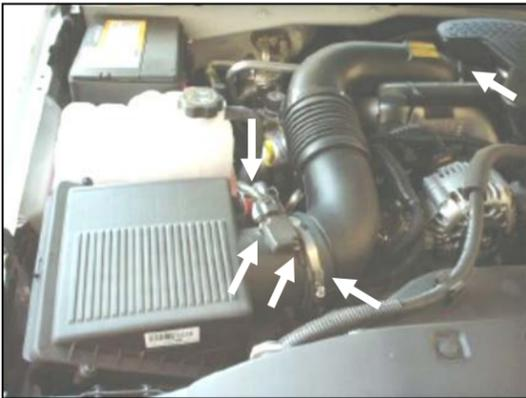
**1. Disconnect the negative battery cable.** Disconnect the Mass Air Flow (M.A.F.) sensor wiring harness. Using the supplied T-20 Security bit, remove the two screws and the M.A.F. sensor from the tube (save the sensor for reuse). Loosen the hose clamps on each end of the factory intake tube assembly.
