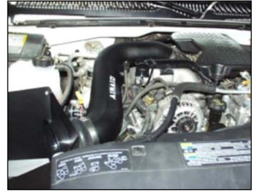
12. Install the Airaid intake tube assembly onto the engine. Install the hump hose end onto the filter adapter first and then slip the coupler end of the tube onto the aluminum intake tube. Adjust for fit, and tighten the hose clamps. (*Note: There should be a gap in between the Airaid intake tube and the air filter adapter.*)
