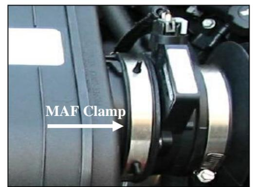
3. Loosen the Mass Air Flow sensor hose clamp. Remove the MAF sensor from the factory air box and temporarily set it aside. Use caution to retain the factory coupler & hose clamp on the MAF.
