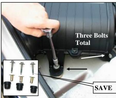
4. Remove the three factory air box hold down bolts, bushings, and grommets. Save them for the Airaid installation.
