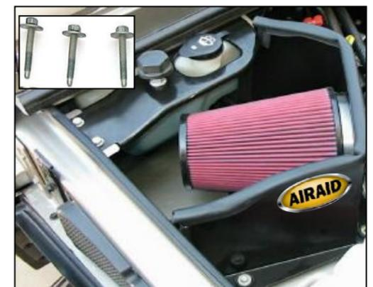
9. Position the Airaid system over the three factory mounting points & secure with the three saved factory bolts removed in step #4. Apply the Airaid Foil Decal onto the Panel as shown.
