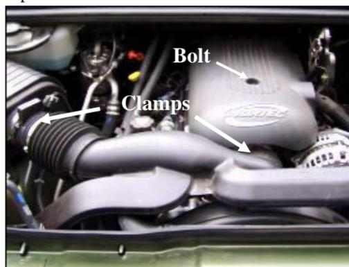
2. Loosen the recessed bolt and remove the beauty cover. Loosen the factory hose clamps on each end of the factory intake tube and remove it from vehicle.
