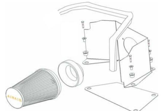
6. Align Cool Air Dam panels (#2, #3) & fasten together with saved grommets and bushings from step #4. Install the filter adapter (#4) using the 3 provided button head bolts (#9) and washers (#10).
