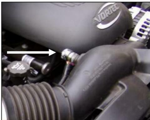
1. **Disconnect negative battery cable.** Remove the factory filter minder and rubber grommet from the factory intake tube, retain for re-installation later in the install.
