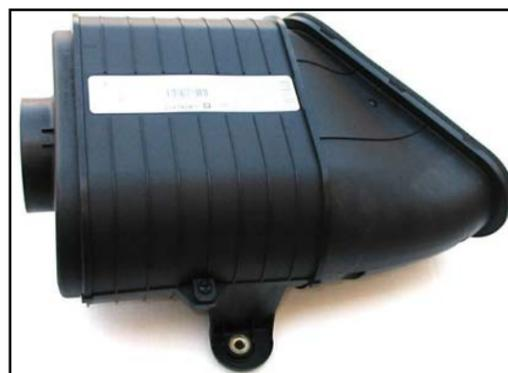
5. Remove the factory air box assembly from the engine compartment.
