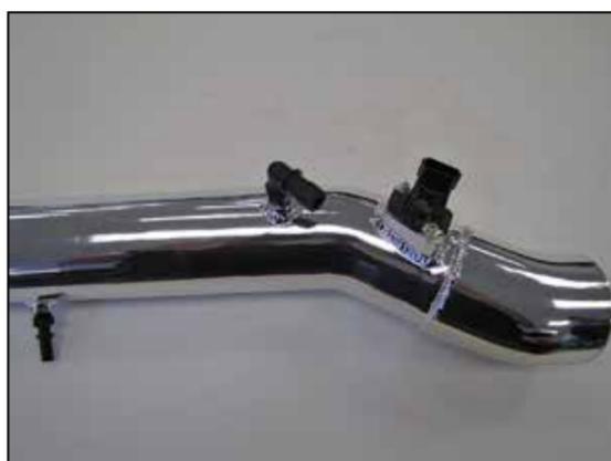
15. Install the 90° vent fitting into the K&N® intake tube as shown.
