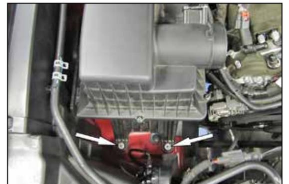
6. Remove the two nuts securing the air filter housing to the inner fender and then remove the housing from the vehicle.
