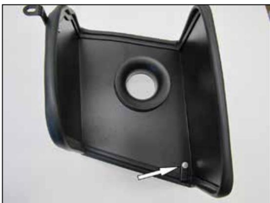
10. Install the provided heat shield mounting bracket (070015) onto the heat shield using the provided hardware and spacer.
