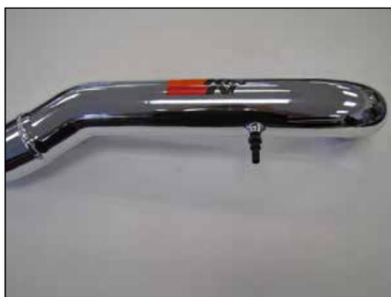
14. Install the quick connect fitting into the K&N® intake tube as shown.
