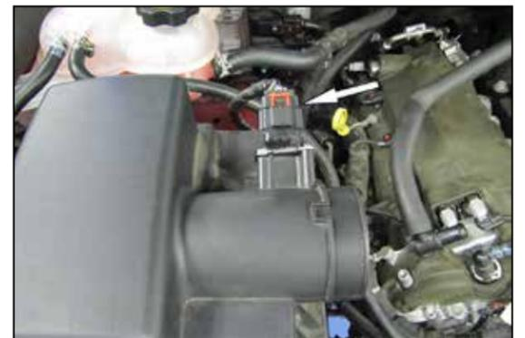
5. Release the red locking tab and then disconnect the mass air sensor electrical connection and unhook the harness from the air filter housing.
