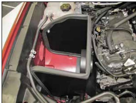
12. Install the heat shield assembly into the vehicle and secure with the factory coolant reservoir nut and air box mounting nut.
