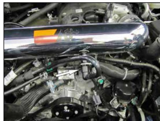
19. Rotate the crank case vent line and fitting so it aligns with the quick connect fitting and then connect.
