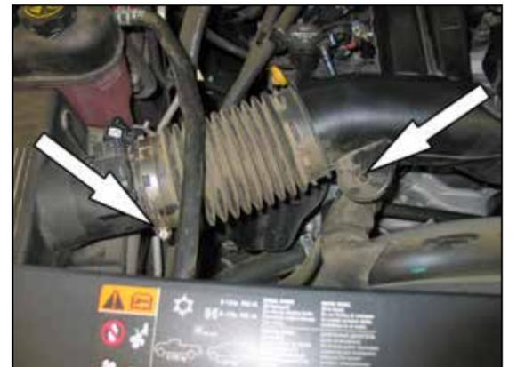
6. Loosen the hose clamp securing the intake tube to the air box housing and disconnect the radiator hose retaining clip from the intake tube. Then remove the intake tube from the vehicle.
