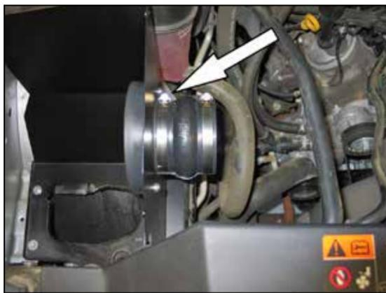
13. Install the provided hump hose (084057) onto the radius adapter and secure with the provided hose clamp.
