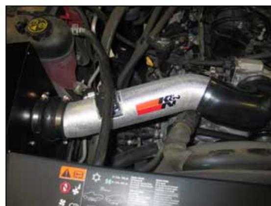
18. Install the K&N intake tube assembly onto the filter adapter and then the throttle body. Adjust the tube and hose for proper fit and then tighten the hose clamps.
