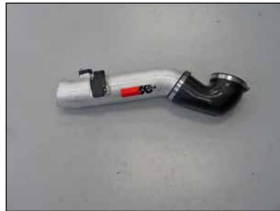
17. Install the provided angle hose onto the K&N intake tube as shown.
