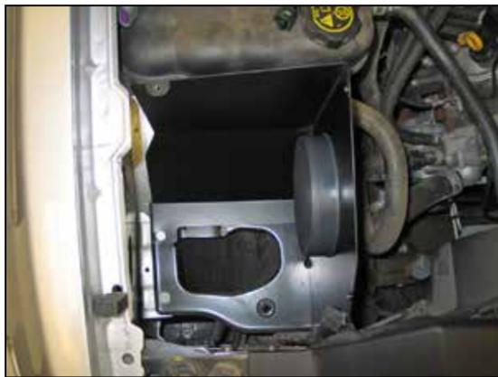
12. Install the heat shield onto the air box mounting plate and secure with the provided hardware to the factory mounting locations.
