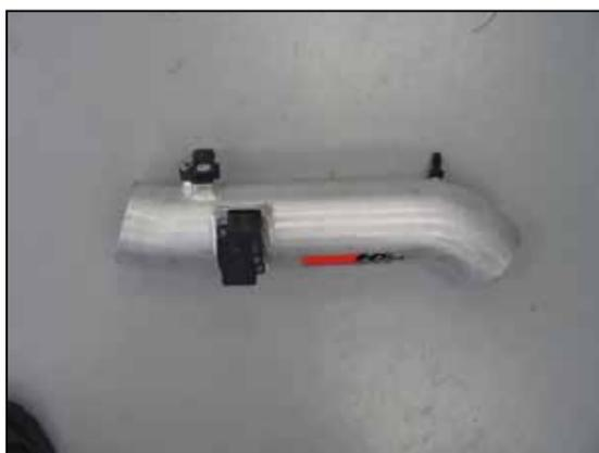
16. Install the sensors into the K&N intake tube and secure with the provided hardware.
