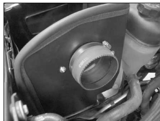
16. Install the silicone hose (08618) onto the filter adapter and secure with the provided hose clamp.
