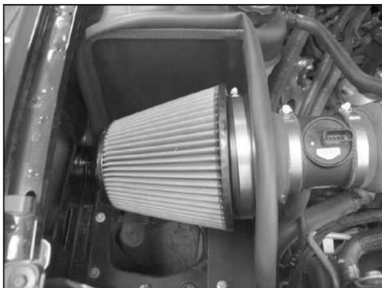
24. Install the K&N® air filter as shown and secure with the provided hose clamp.
