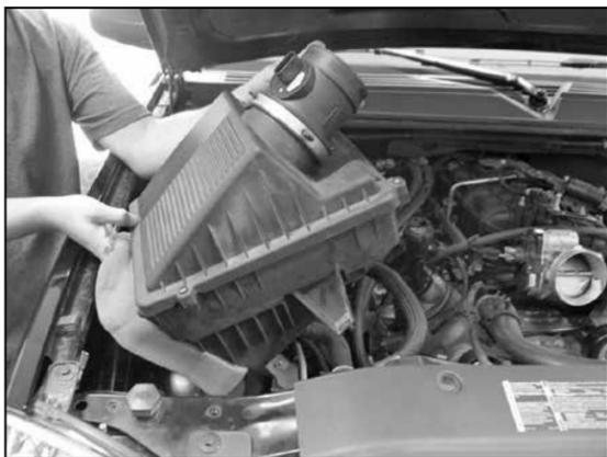
7. Pull firmly upwards to release the air cleaner assembly from the mounting tray grommets, and then remove the assembly as shown.
