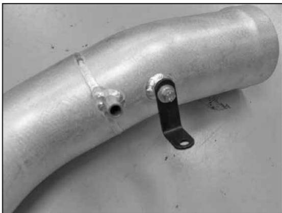
20. Install the "L" bracket (070812) onto the K&N® intake tube with the provided hardware as shown.
