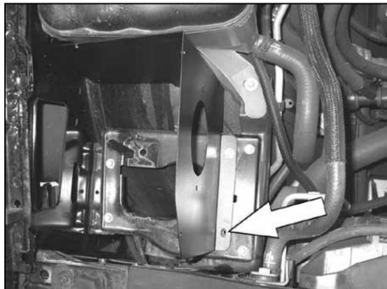
12a. On vehicles that are not equipped with the front airbox mounting grommet and hole, install the heat shield assembly as shown. Then, use a marker to mark the mounting plate through the heat shield mounting hole.
