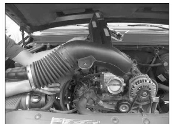
6. Loosen the hose clamps, which secure the stock intake tube to the throttle body and mass air sensor and then remove the intake tube from the vehicle.
