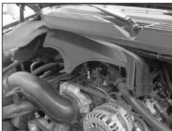
3. Lift up on the front of the engine cover to disengage from the mounting grommets. Then pull forward and remove the engine cover from the engine as shown.
