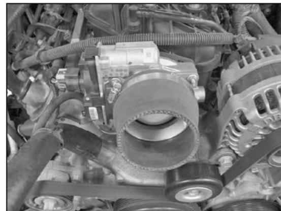
17. Install the silicone (08050) hose onto the throttle body and secure with the provided hose clamp.
