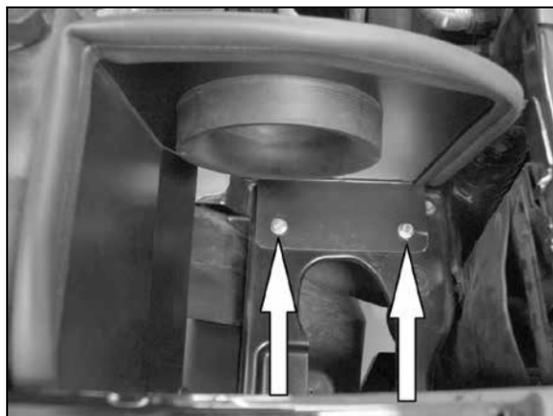
14. Install the heat shield assembly onto the airbox mounting tray and secure to the 5/16" inserted nuts with the provided hardware as shown.
