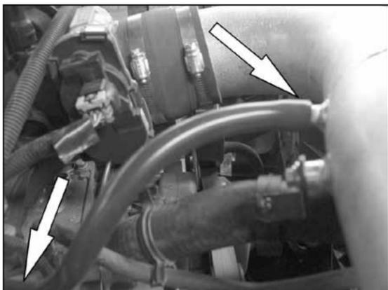
23. Install the provided crank case vent hose onto the valve cover and then onto the K&N® intake tube as shown.
