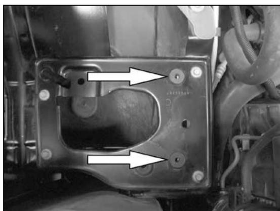
13. Install the two 5/16" inserted nuts into the airbox mounting tray as shown.
