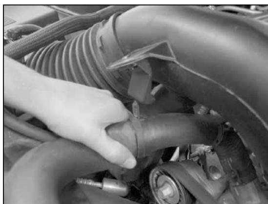
4. Unhook the radiator hose mount from the intake tube.
