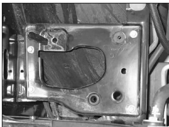
12b. Remove the heat shield assembly and drill a 5/8" hole through the marked location from step #12a.
