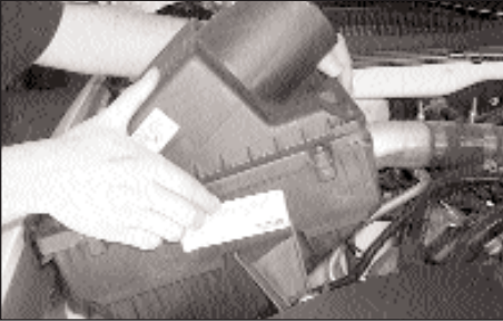
7. Pull firmly upwards to remove the stock air cleaner as shown. NOTE: K&N recommends that you do not discard your factory air intake.
