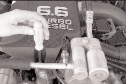
3. On 2001 models remove the 8mm bolt that secures the engine cover, then remove the cover.
