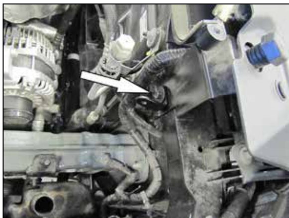
12. Install the provided heat shield mounting bracket (064323) onto the core support and secure with the factory bolt removed in the previous step.
