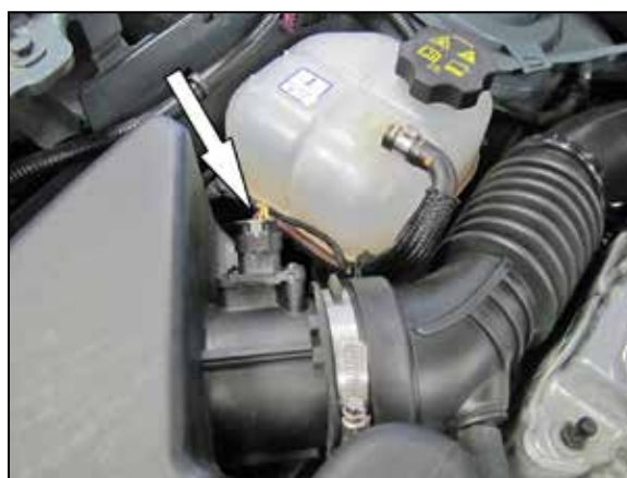
4. On vehicles equipped with a humidity sensor, disconnect the humidity sensor electrical connection.
