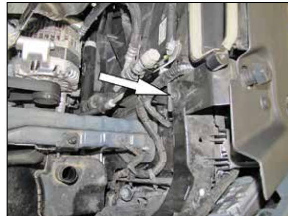
20. On vehicle equipped with a humidity sensor, install the sensor into the K&N® intake tube. On all other vehicles install the provided gasket onto the block off plate and install the block off plate onto the K&N® intake tube.
