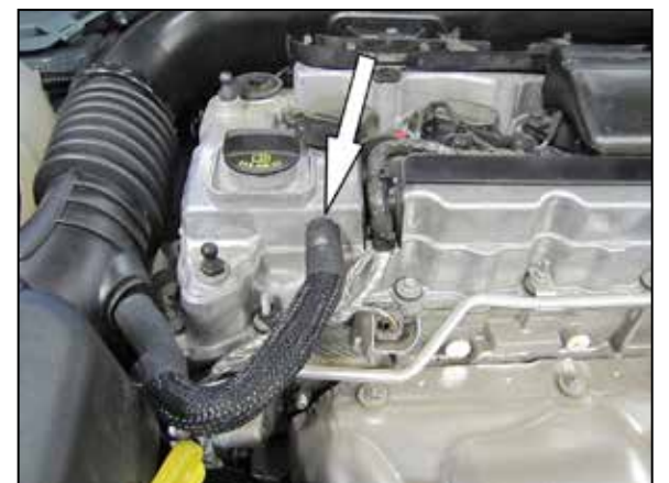
5. Disconnect the crank case vent hose from the valve cover port.
