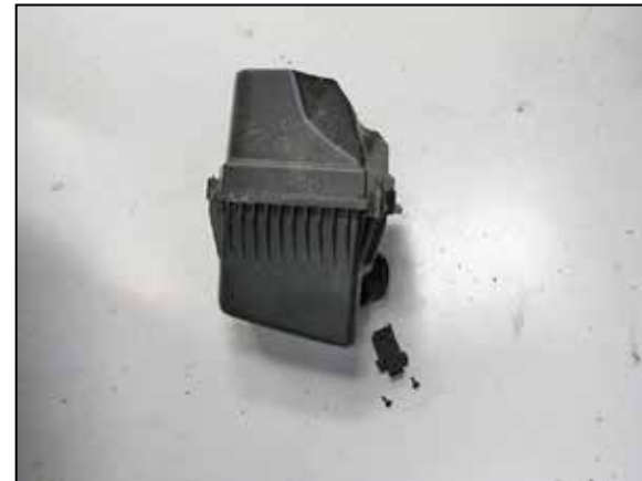
19. If the vehicle is equipped with a humidity sensor, remove the humidity sensor from the factory air filter housing.
