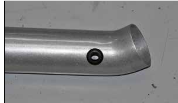
21. Install the provided grommet into the K&N® intake tube.
