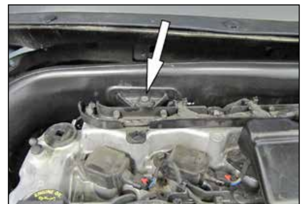
6. Remove the bolt securing the intake tube to the valve cover.
