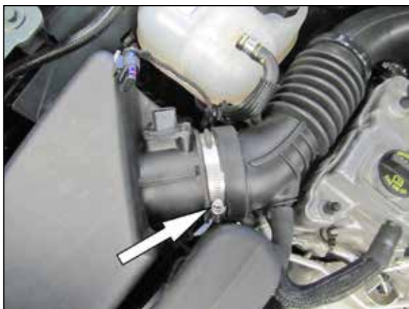
7. Loosen the hose clamp securing the intake tube to the air filter housing.
