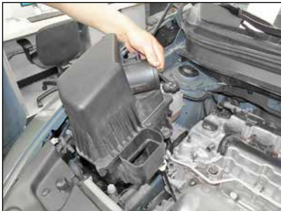
10. Lift up the air filter housing to dislodge it from the mounting grommets and remove it from the vehicle.
