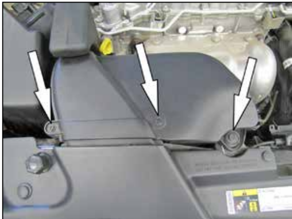
9. Remove the three bolts that secure the fresh air intake scoop and then lift up and remove the scoop from the vehicle.
