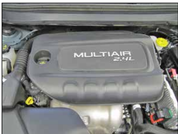
2. Lift up and remove the decorative engine cover and remove it from the vehicle.
