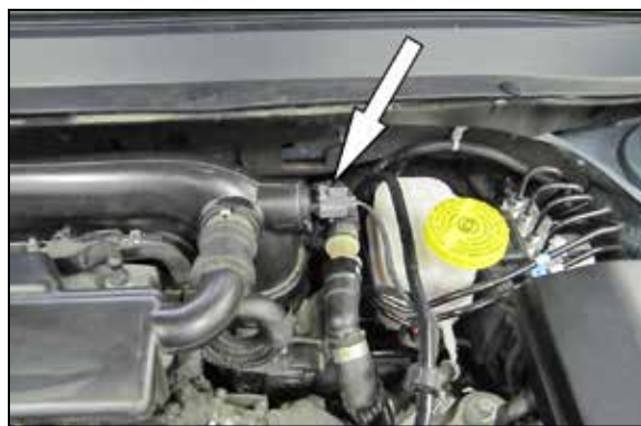
3. Disconnect the inlet air temperature sensor electrical connection.
