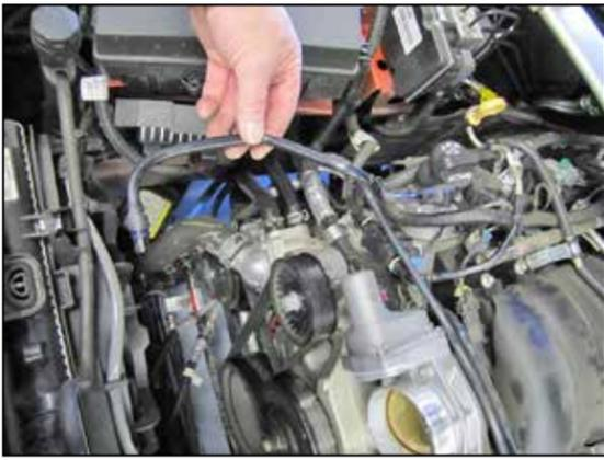
7. Rotate the crank case vent tube 180°, then release the retainer at the valve cover port and the remove the crank case vent tube.
