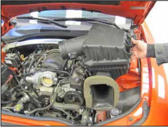
9. Lift up and remove the air box from the vehicle.
