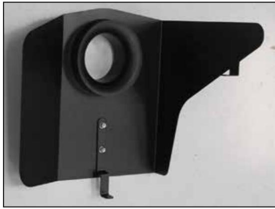
12. Install the filter adapter onto the heat shield and secure with the provided hardware.
