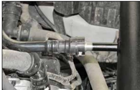
20. Connect the crank case vent hose to the quick disconnect fitting on the K&N® intake tube.
