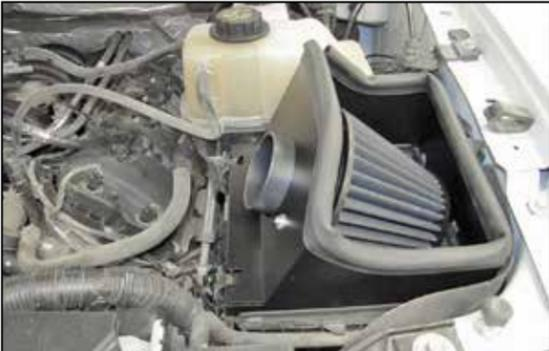
13. Install the heat shield/filter assembly onto the lower air box and secure with the factory air box retaining clips.
