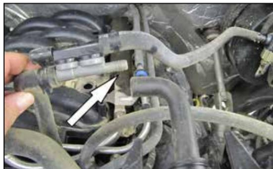
4. Disconnect the EVAP hose from the check valve as shown.
