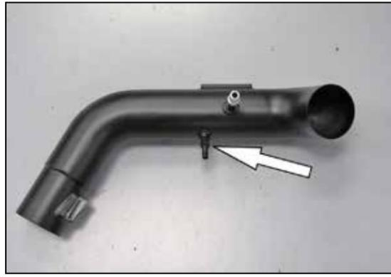
16. Install the provided 3/8" NPT hose fitting into the K&N® intake tube as shown.
