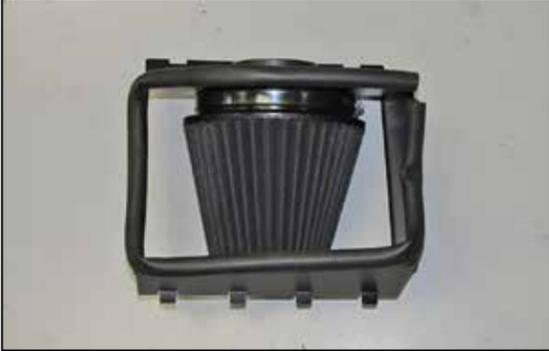
11. Install the air filter onto the filter adapter and secure with the provided hose clamp.
