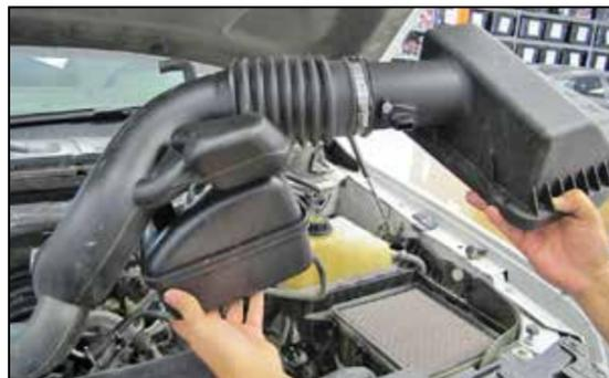
6. Release the three clips securing the upper air box housing to the lower housing and then remove the intake tube/upper air filter housing and air filter from the vehicle.
