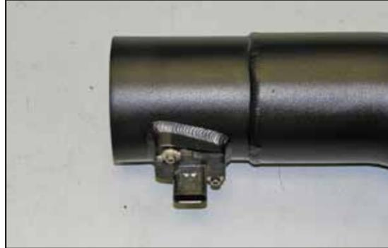
18. Install the mass air sensor into the K&N® intake tube and secure with the provided hardware.
