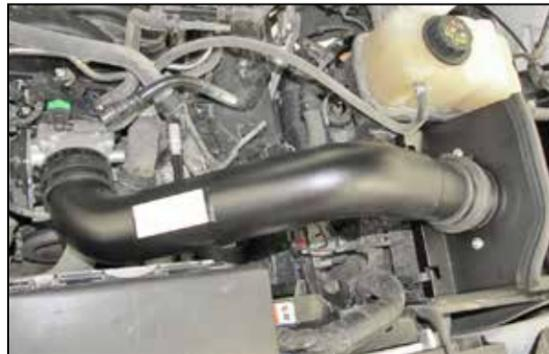
19. Install the intake tube assembly into the silicone hose at the filter adapter and then into the silicone hose on the throttle body and secure with the provided hose clamps.
