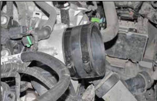
14. Install the provided coupling hose (08630) onto the throttle body and secure with the provided hose clamp.
