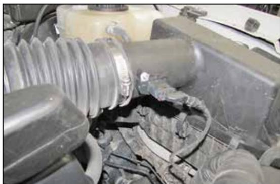
2. Release the red locking tab and then disconnect the mass air sensor electrical connection.
