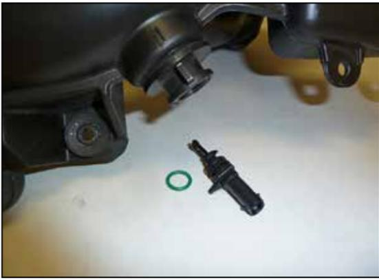
7. Remove the temp sensor from the factory intake tube by gently lifting the tab and rotating the sensor counter clockwise. Once the sensor is removed, remove the sealing O ring from the sensor.
