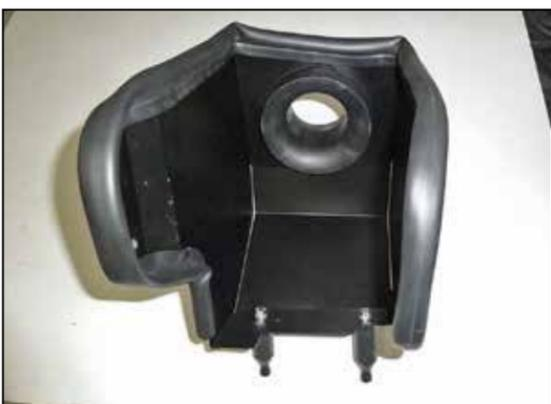
10. Install the provided edge trim onto the heat shield as shown, some trimming of the edge trim will be necessary. Install the two provided mounting studs onto the heat shield and secure with the provided hardware.
