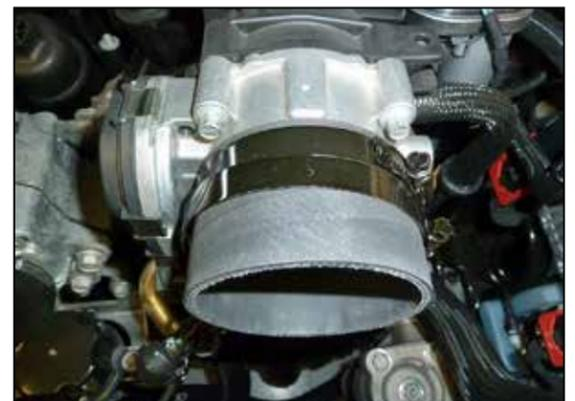
6. Install the provided coupler (08690) onto the throttle body and secure with the provided hose clamp.
