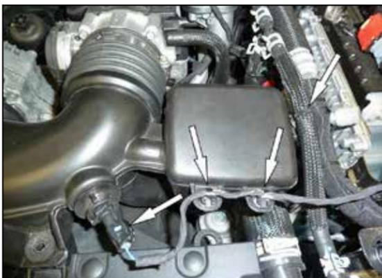
2. Disconnect the inlet air temperature sensor connection and unhook the wiring harness from the intake plenum. Unhook the coolant by-pass hose from the intake plenum and loosen the hose clamp that secures the tube to the throttle body.
