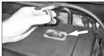
5. On set-up "A" vehicles, remove the cap on top of the the air box and unscrew the allen head bolt underneath.
