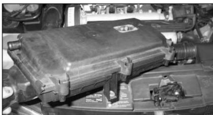
6. On set-up "A" vehicles, remove the screw securing the intake hose to the air box. Remove the bolt securing the air box to the vehicle, then, remove the air box. On 1.4L models, go to step 9; on 1.6L models, go to step 11.
