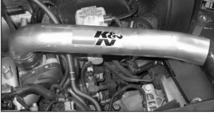
16. Align the tube for fit and clearance, then, firmly tighten the #275 barrel clamp and bracket securing hardware.
