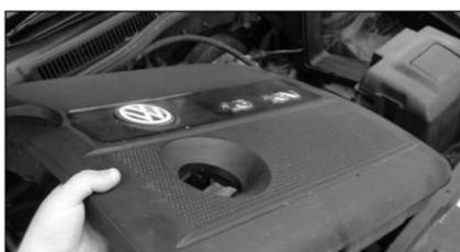
8. On set-up "B" vehicles, remove the complete air box/ engine cover from the vehicle by pulling it out of its grommets and go to step 11.
