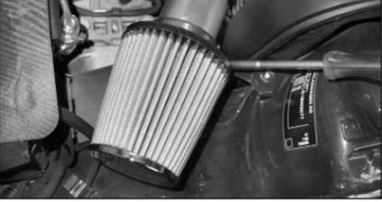
17. Fit the filter onto the tube using the #40 hose clamp supplied.
