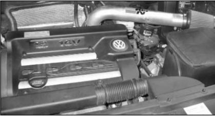
21. On set-up "A" vehicles (set-up "B" vehicles go to step 23), re-install the engine cover using its original bolts as shown.
