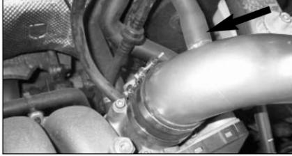
19. Fit the other end of the breather hose onto the tube.
