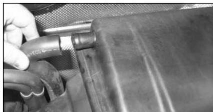
4. On set-up "A" vehicles, remove the breather hose from the air box as shown.
