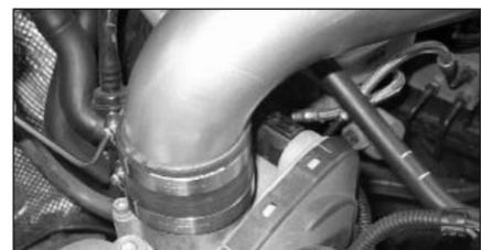
14. Fit the tube into the silicone sleeve using a #275 barrel clamp supplied (do not fully tighten yet).
