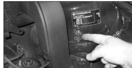
12. Screw the rubber vibration stud into the under side of the threaded support bracket on the suspension turret as shown.
