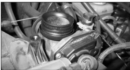
10. On 1.4L vehicles, fit the previously removed rubber sleeve onto the throttle body as shown.
