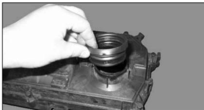
9. On 1.4L vehicles (1.6L vehicles, go to step 12), remove the rubber sleeve from the air box.
