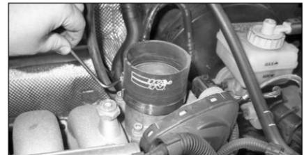
11. Fit the appropriate silicone sleeve and barrel clamp on the throttle body as shown (to tighten, use the 9/64" Allen wrench supplied). On 1.4L vehicles, use the stepped silicone sleeve and the #250 barrel clamp; on 1.6L vehicles, use the straight silicone sleeve and a #275 barrel clamp.
