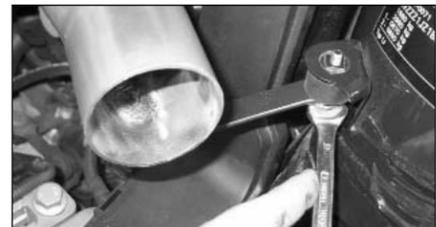
15. Secure the bracket to the rubber vibration stud using an M6 nylock nut and washer supplied (do not fully tighten yet.)
