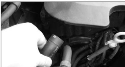
7. On set-up "B" vehicles, remove the breather hose from the side of the air box as shown.
