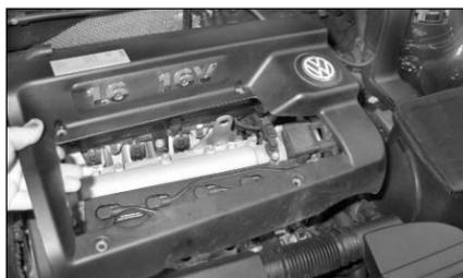
3. On set-up "A" vehicles, unbolt and remove the engine cover from the vehicle.
