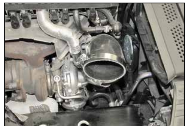
6. Install the provided turbo inlet hose (08490) onto the turbo and secure with the provided hose clamp. NOTE: Do not completely tighten at this time.
