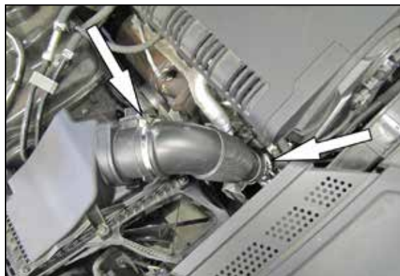
4. Loosen the hose clamps securing the factory intake tube and then remove the intake tube from the vehicle.
