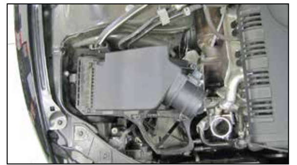
5. Lift up the complete air filter housing to dislodge it from the mounting studs and then remove it from the vehicle.
