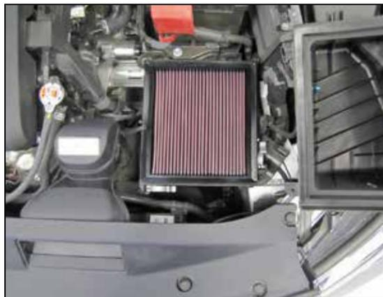
3. Release the clips that secure the upper air filter housing and then remove the upper housing from the lower housing. Replace the factory air filter with the provided K&N® air filter, reinstall the lid and secure with the factory retaining clips.
