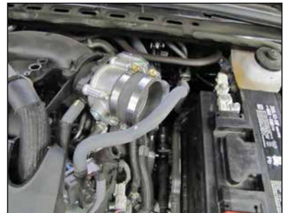
5. Install the provided coupler (08690) onto the throttle body and secure with the provided hose clamp.
