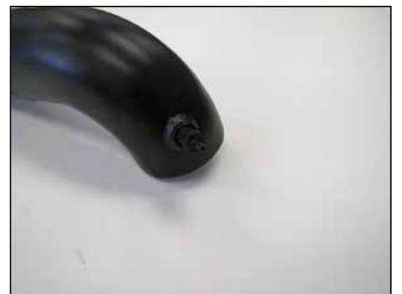
6. Install the provided vent fitting into the K&N® intake tube as shown.
